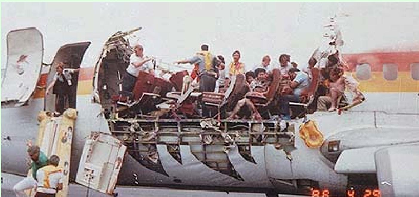
*A section of the upper fuselage of a Boeing 737-200 was torn away at 24,000 feet
