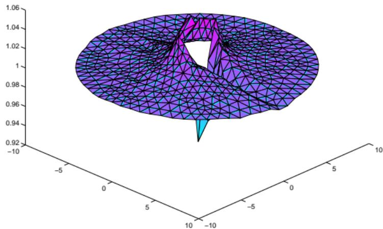
Figure: Pressure distribution around shapes of maximal drag.
