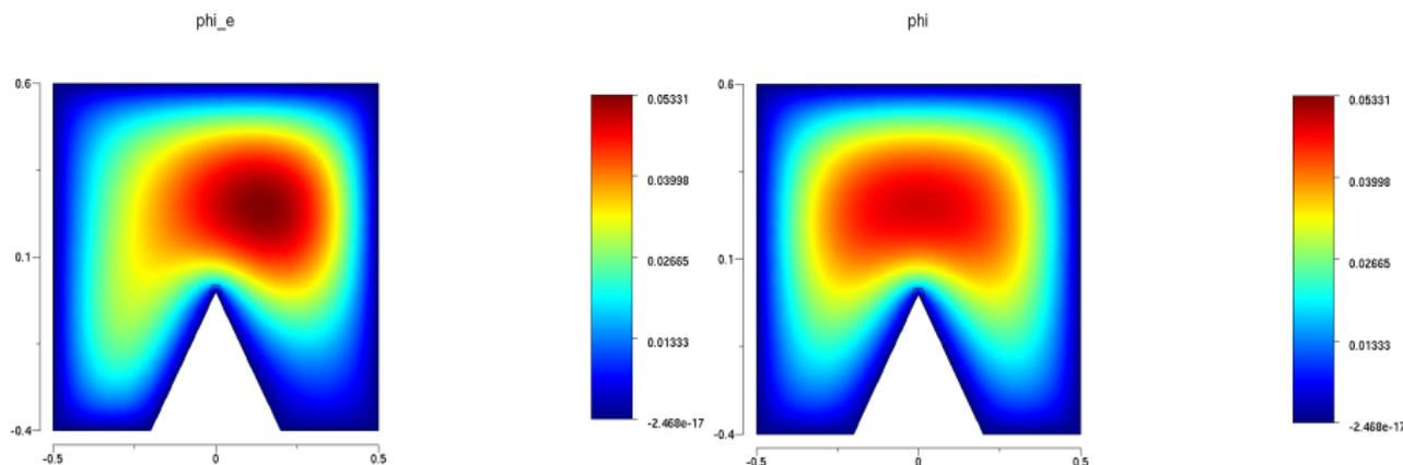
$$-\Delta\phi_e = \rho_e; \quad -\Delta\phi = \rho \propto e^{\phi_e - \phi}; \quad \phi_e = \phi = 0 \text{ on } \Gamma.$$
