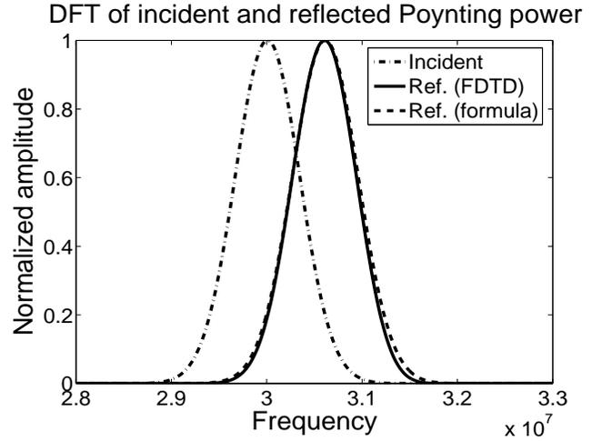
Fig. 3. Reversed Doppler shift in two-dimensional simulation.
