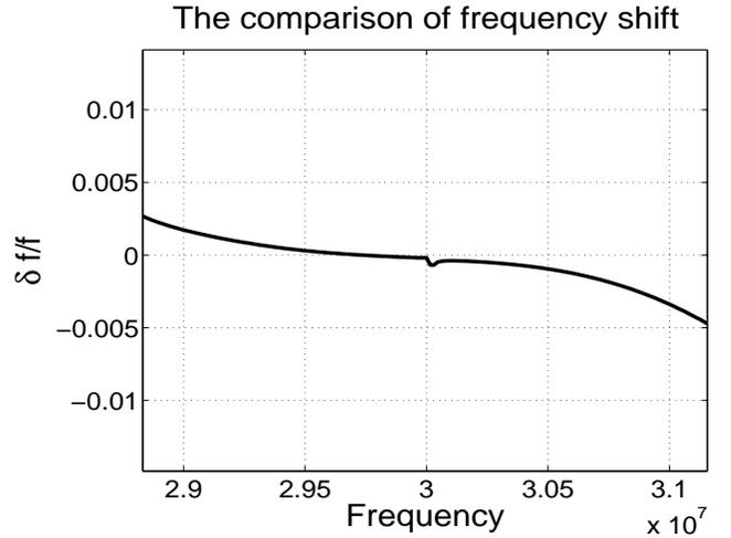
Fig. 4. Comparison between the FDTD simulation and theoretical prediction.
