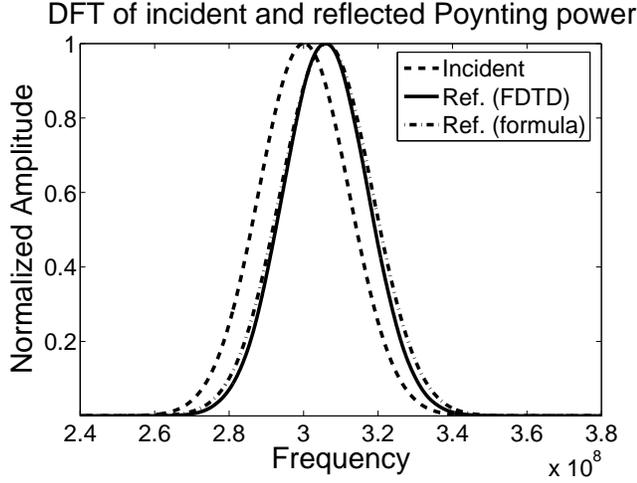
Fig. 2. Reversed Doppler shift in one-dimensional simulation.
