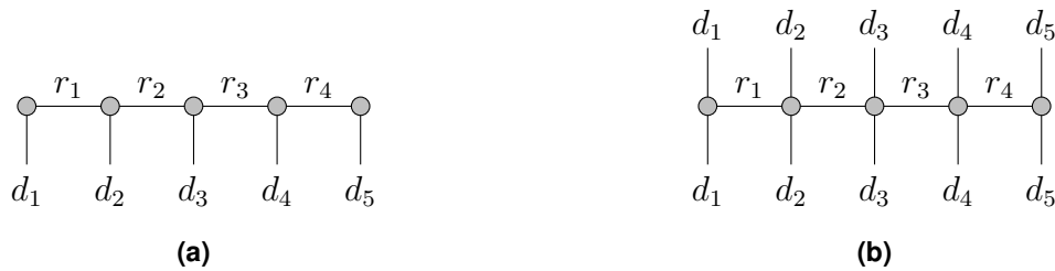
Figure 1: Graphical representation of tensor trains: Tensors are depicted as circles with different arms indicating the set of free indices. (a) Tensor of order 5 in TT format, the first and the last core are matrices, the other cores are tensors of order 3. (b) Linear operator in TT format, the first and the last core are tensors of order 3, the other cores are tensors of order 4. In both cases, arms corresponding to first and last TT ranks are omitted since r_0 = r_5 = 1 .
