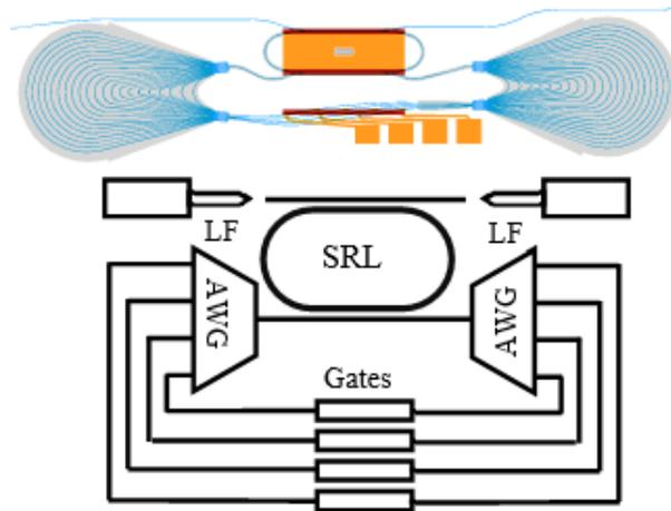
Figure 1: The mask layout (top) and the schematic representation (bottom) of the considered SRL with four branches of the FOF. AWG: Arrayed Waveguide Grating, LF: Lensed Fiber.
