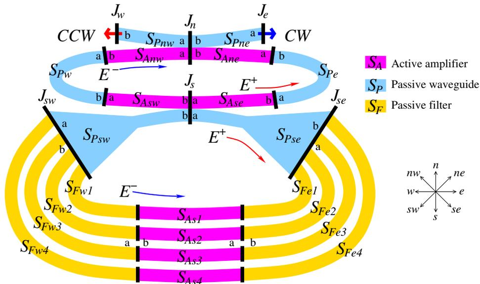
Figure 4: Schematic representation of the simulated integrated SRL with four branches of filtered and amplified bidirectional optical feedback. Black segments and colored frames indicate different junctions and sections of the SRL. Red and blue arrows show propagation directions and the emission of the CCW and CW fields  $E^+$  and  $E^-$ , respectively.
