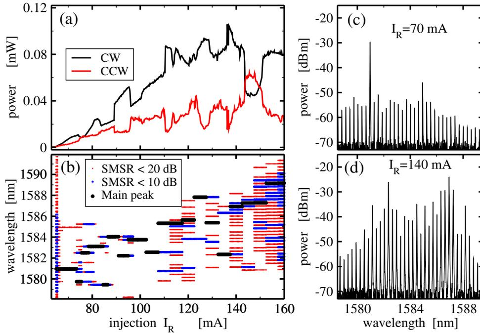
Figure 2: Measurements of the SRL device with uninjected FOF. Intensities of the emitted CW (black) and CCW (red) fields (a) and main lasing wavelengths of the CCW field (b) as functions of the total ring laser current  $I_R$ . Large, medium, and small bullets in panel (b) represent the main spectral peak and all side peaks suppressed by less than 10 dB and less than 20 dB, respectively. (c) and (d): optical spectrum of the CW field at  $I_R = 70$  mA and 140 mA, respectively.
