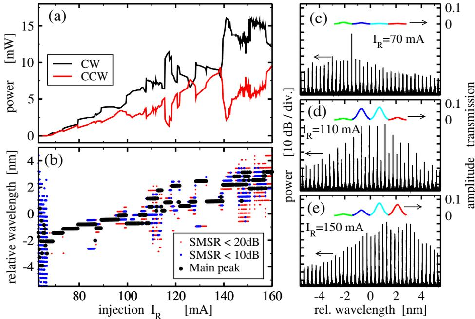
Figure 5: Simulated performance of the SRL with uninjected FOF. (a) and (b): the same as in experimental figures 2(a) and (b). (c)–(e): optical spectra of the CW emission at  $I_R = 70\text{ mA}$ ,  $110\text{ mA}$ , and  $150\text{ mA}$ . Corresponding instantaneous field amplitude transmission spectra for all four FOF branches are plotted on the top of these panels.
