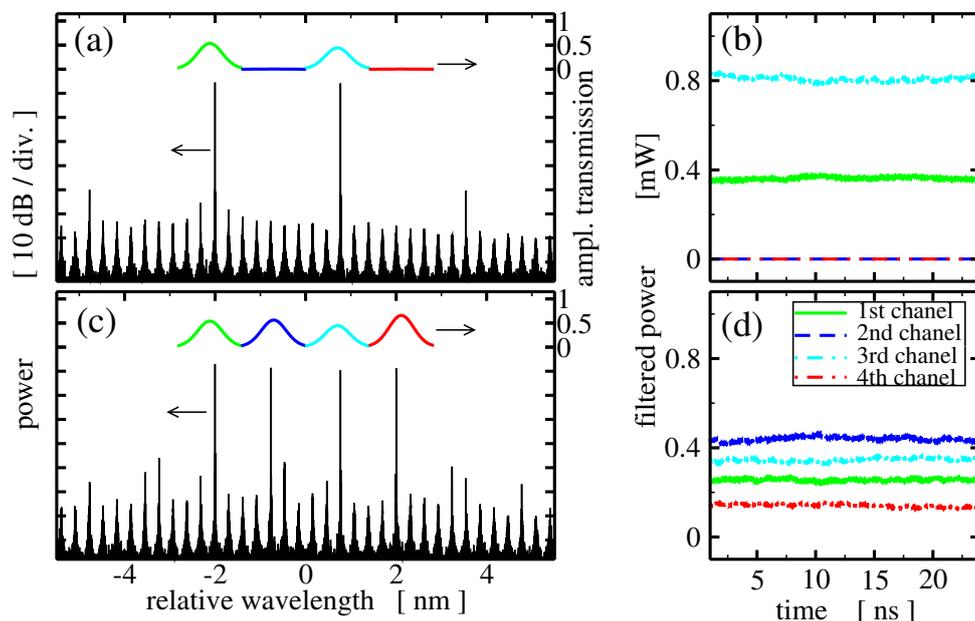
Figure 8: Simulated stable multicolor lasing of the SRL with  $I_R = 85$  mA and the gate currents  $(I_1, I_2, I_3, I_4) = (29, 0, 18, 0)$  mA (above) and  $(29, 32, 18, 49)$  mA (below). (a) and (c): optical spectra of the CW emission (black) and transmission spectra for all four FOF branches (colored). (b) and (d): corresponding time-traces of the CW field after four digital filters centered at  $\bar{\lambda}_1, \dots, \bar{\lambda}_4$ .
