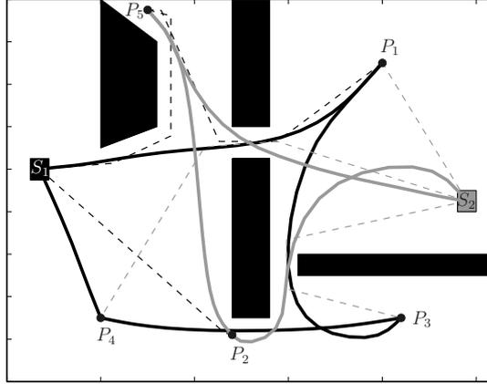
FIGURE 3. The tours  $T^1 = (S_1, P_1, P_3, P_4, S_1)$  and  $T^2 = (S_2, P_2, P_5, S_2)$  with exact trajectories. The dashed lines are approximated trajectories which were not considered in a tour yet.
