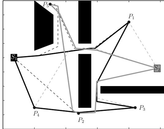
FIGURE 2. The tour  $T^1$  based on the approximated trajectories is given by  $(S_1, P_1, P_3, P_4, S_1)$  and represented by the black bold line. The tour of robot  $R_2$  is  $T^2 = (S_2, P_2, P_5, S_2)$  and depicted in grey. The dashed black, resp. grey, lines are the approximated trajectories related to the arcs in  $A_1$ , resp.  $A_2$ , which do not belong to the tour  $T^1$ , resp.  $T^2$ .
