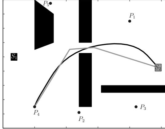
FIGURE 1. The black curve is the exact trajectory of robot  $R_2$  which moves from  $S_2$  to  $P_4$ . The corresponding approximated trajectory is the sequence of line segments illustrated in grey.
