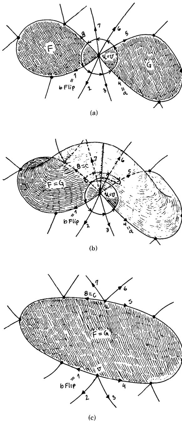
Fig. 13. The effect of *splice*: Adding or removing a cross-cap. (a)  $a \text{ Org} = b \text{ Flip Org}$ ,  $a \text{ Left} = b \text{ Left}$ . (b)  $a \text{ Org} = b \text{ Flip Org}$ ,  $a \text{ Left} = b \text{ Left}$ ;  $c \text{ Left} = b \text{ Flip Left}$ ,  $c \text{ Org} = b \text{ Org}$ . (c)  $c \text{ Left} = b \text{ Flip Left}$ ,  $c \text{ Org} \neq b \text{ Org}$ .
