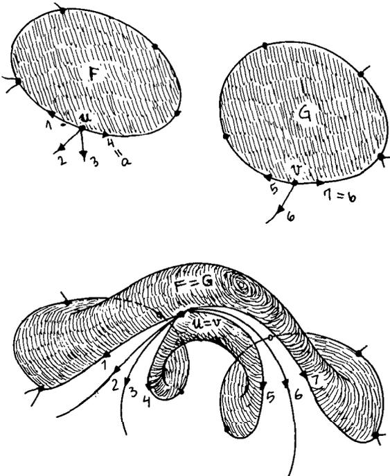
Fig. 11. The effect of Splice: Changing the connectivity of the manifold. (a)  $a \text{ Org} \neq b \text{ Org}$ ,  $a \text{ Left} \neq b \text{ Left}$ . (b)  $a \text{ Org} = b \text{ Org}$ ,  $a \text{ Left} = b \text{ Left}$ .
