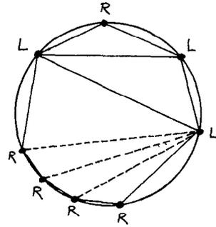
Fig. 16. Triangulating a face of the Delaunay.
