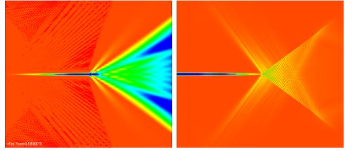
Fig. 2. CW state: Photon density of forward (left) and backward field (right)
