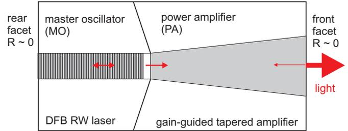
Fig. 1. Top view of a MOPA device consisting of a DFB Master Oscillator (MO) and a tapered Power Amplifier (PA).
