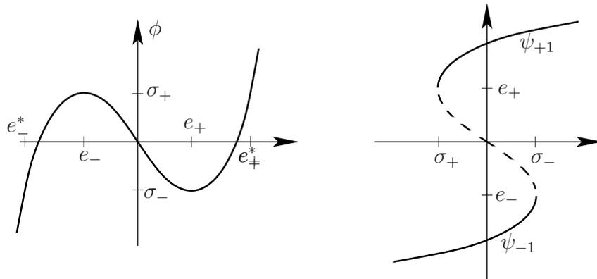
Figure 2.1: Left: Non-monotone stress-strain relation. Right: Two branches  $\psi_{+1}$  and  $\psi_{-1}$  of the strain-stress relation
