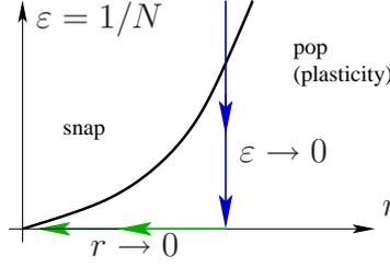
Figure 3.1: Schematic phase diagram in the space of small parameters indicating location of the ‘popping’ domain which we associate with rate-independent plasticity response.
