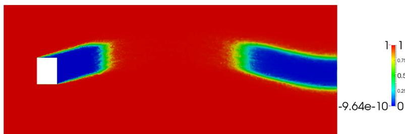
**Fig. 13** The 3d example: The slice at  $z = 1$  of the approximation obtained using the BJK method. It took 1117 iterations for the Euclidean norm of the residual in the damped fixed point algorithm to be less than the tolerance of  $10^{-6}$ .
