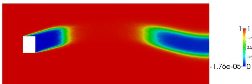
**Fig. 14** The 3d example: The slice at  $z = 1$  of the approximation obtained by the Kuzmin limiter. It took 70 iterations for the Euclidean norm of the residual in the damped fixed point algorithm to be less than the tolerance of  $10^{-6}$ .
