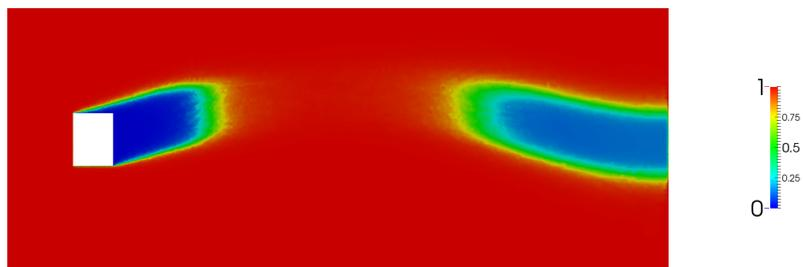
**Fig. 12** The 3d example: The slice at  $z = 1$  of the approximation obtained using the BBK method. It took 166 iterations for the Euclidean norm of the residual in the damped fixed point algorithm to be less than the tolerance of  $10^{-6}$ .
