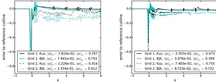
**Fig. 5** Hemker example: Errors to the cutline at  $y = 1$ , left level 3 (nearly 10000 d.o.f.s), right level 5 (nearly 150000 d.o.f.s).
