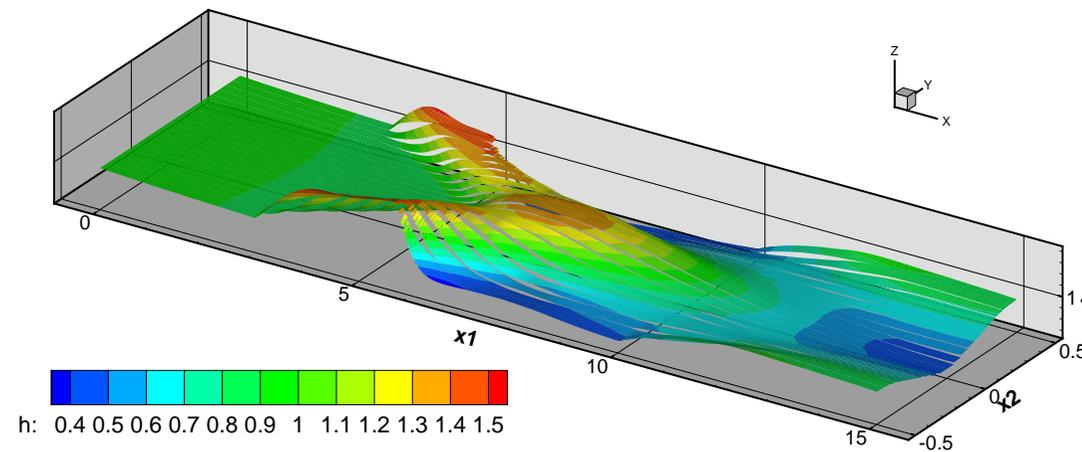
Flow depth  $h$  of water-sand mixture in a contraction
