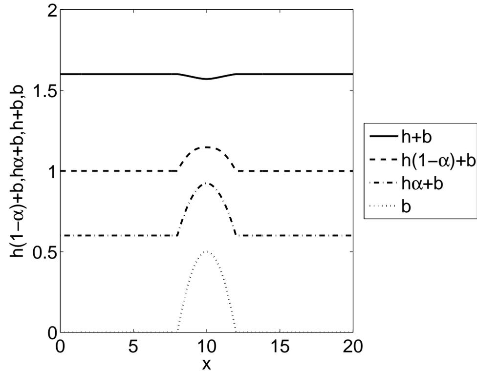
Steady-state solution for a subcritical two-phase flow (320 cells).
