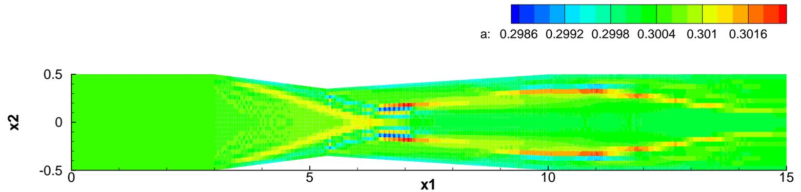
Particle volume fraction  $\alpha$  of water-sand mixture in a contraction
