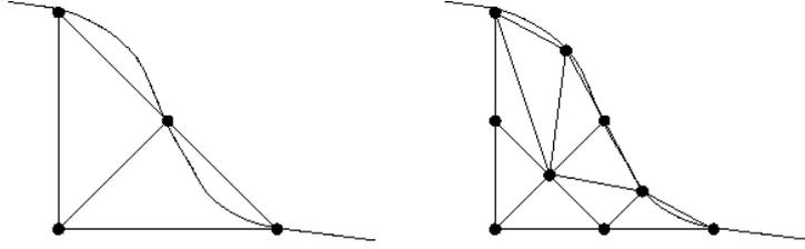
Figure 7.1: Approximation of the boundary by the finite element mesh.
