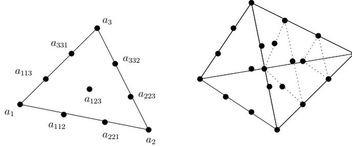
Fig. B.5 The finite element  $P_3(K)$ .
