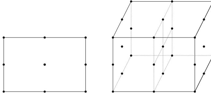
Fig. B.8 The finite element  $Q_2(K)$ .
