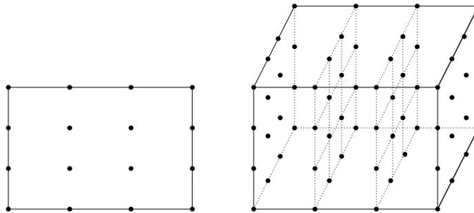
Fig. B.9 The finite element  $Q_3(K)$ .
