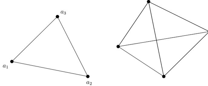
**Fig. B.3** The finite element  $P_1(K)$ .
