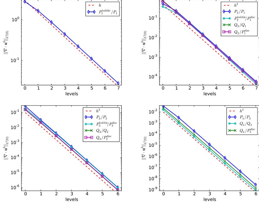
**Fig. 3.4** Example 3.27. Convergence of the errors  $\|\nabla \cdot \mathbf{u}^h\|_{L^2(\Omega)}$  for different discretizations with different orders  $k$ . In the top right and bottom left pictures, the magenta line is on top of the green line.
