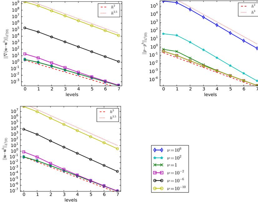
**Fig. 3.7** Example 3.29. Convergence of the errors for the scaled Stokes problem and the  $P_2/P_1$  pair of finite element spaces.
