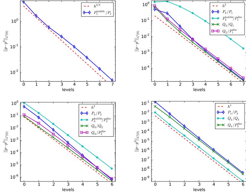
**Fig. 3.5** Example 3.27. Convergence of the errors  $\|p - p^h\|_{L^2(\Omega)}$  for different discretizations with different orders  $k$ .
