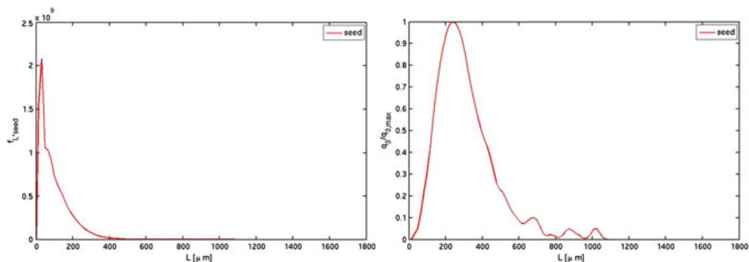
Figure 3.  $f_{L,seed}(L)$  at the inlet (left) and the normalised volume fraction of the PSD at the inlet (right).
