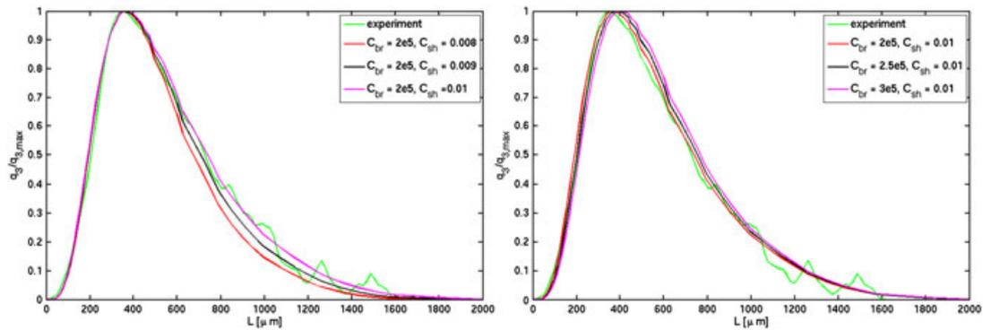
Figure 7. Flow rate  $V_f = 30$  ml/min; space–time-averaged normalised volume fraction at the outlet for different parameters  $C_{br}$  and  $C_{sh}$ .
