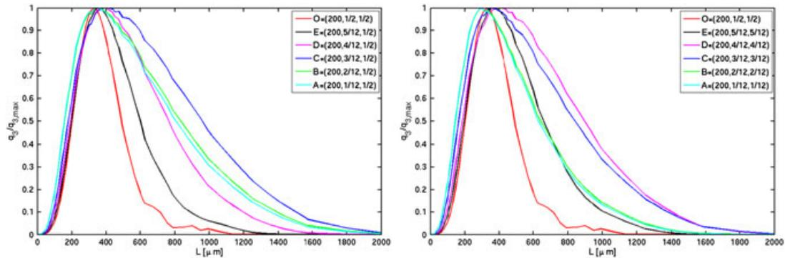
Figure 9. Flow rate  $V_r = 30$  ml/min; time-averaged normalised volume fraction at the outlet for different nodes,  $C_{br} = 2 \cdot 10^5$  and  $C_{sh} = 0.01$ .
