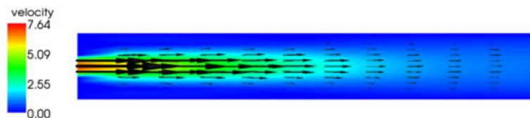
Figure 6. Experiment with flow rate  $V_r = 30$  ml/min; cut of the stationary velocity field at the inlet of the channel.
