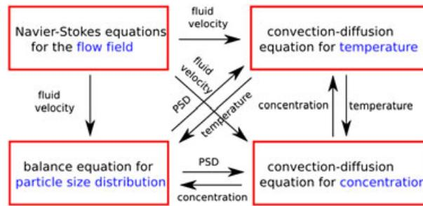
Figure 1. Couplings of the equations in the population balance system for the urea synthesis.
