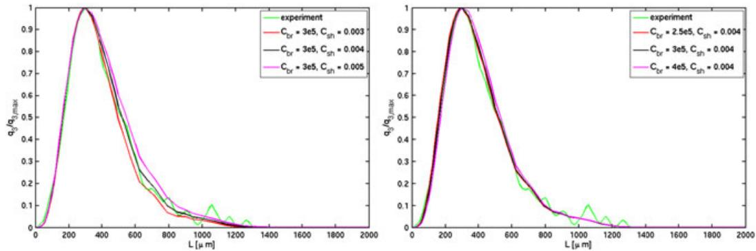
Figure 11. Flow rate  $V_f = 90$  ml/min; space-time-averaged normalised volume fraction at the outlet for different parameters  $C_{br}$  and  $C_{sh}$ .
