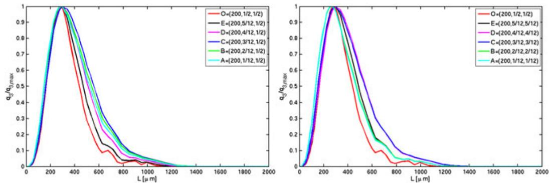
Figure 13. Flow rate  $V_f = 90$  ml/min; time-averaged normalised volume fraction at the outlet for different nodes,  $C_{br} = 3 \cdot 10^5$  and  $C_{sh} = 0.004$ .
