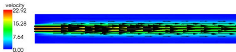
Figure 10. Experiment with flow rate  $V_r = 90$  ml/min; cut of the stationary velocity field at the inlet of the channel.
