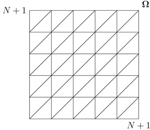
**Figure 4.3:** Triangulation of  $\Omega$  with  $(N - 1)^2$  inner nodes for the unstable  $\mathbf{P}_1/P_0$ -finite element
