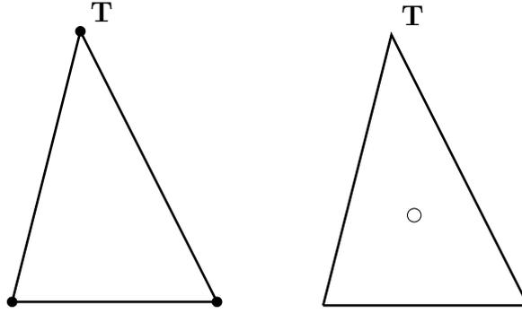
**Figure 4.2:** Elements of the triangulation  $\mathcal{T}_h$  with the local degrees of freedom represented as filled circles for the velocity (left) and with the local degree of freedom pictured by a circle for the pressure (right), for the  $\mathbf{P}_1/P_0$  element.
