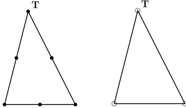
**Figure 4.8:** Elements of the triangulation  $\mathcal{T}_h$  with the local degrees of freedom represented as filled circles for the velocity (left) and with the local degrees of freedom pictured by circles for the pressure (right), for the stable Taylor–Hood element  $\mathbf{P}_2/P_1$ .
