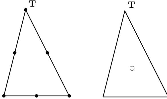
**Figure 4.7:** Elements of the triangulation  $\mathcal{T}_h$  with the local degrees of freedom represented as filled circles for the velocity (left) and with the local degree of freedom pictured by a circle for the pressure (right), for the stable  $\mathbf{P}_2/P_0$ -element.
