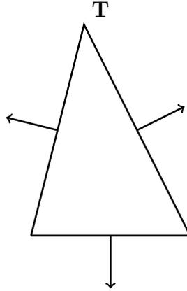
**Figure 5.1:** An element of the triangulation  $\mathcal{T}_h$  with the local degrees of freedom represented as normal vectors in the face barycenters for the velocity, for the Raviart–Thomas space  $\mathbf{V}_h^{\text{RT}}$ .
