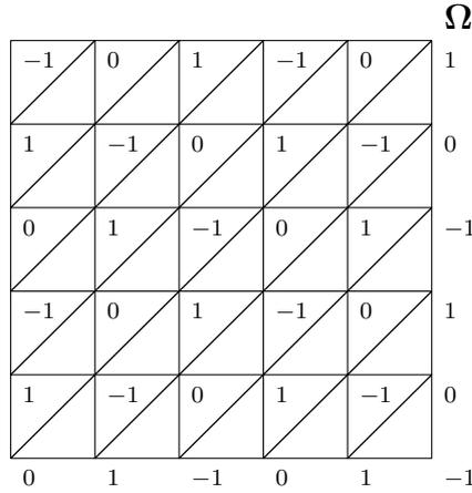
**Figure 4.4:** A spurious pressure mode for  $\mathbf{P}_1/P_1$  with nodal pressure values.
