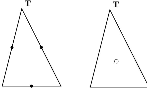
**Figure 4.11:** Elements of the triangulation  $\mathcal{T}_h$  with the local degrees of freedom represented as filled circles for the velocity (left) and with the local degree of freedom pictured by a circle for the pressure (right), for the nonconforming Crouzeix–Raviart element  $\mathbf{P}_1^{\text{nc}}/P_0$ .
