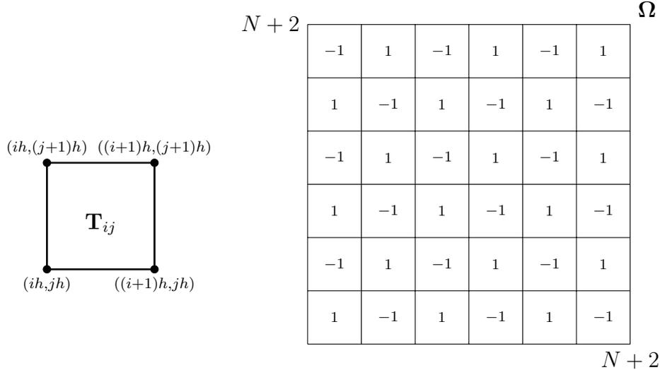
**Figure 4.5:** Checkerboard-instability: A spurious pressure mode for  $\mathbf{Q}_1/Q_0$  with elementwise pressure values.
