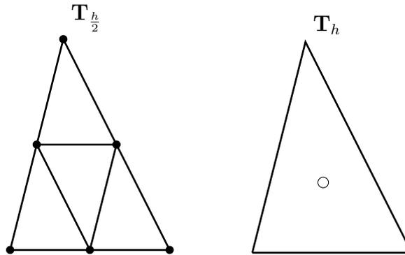
**Figure 4.6:** Elements of the triangulations  $\mathcal{T}_{\frac{h}{2}}$  with the local degrees of freedom represented as filled circles for the velocity (left) and  $\mathcal{T}_h$  with the local degree of freedom pictured by a circle for the pressure (right), for the stable  $\mathbf{P}_1$ -iso- $\mathbf{P}_2/P_0$ -element.
