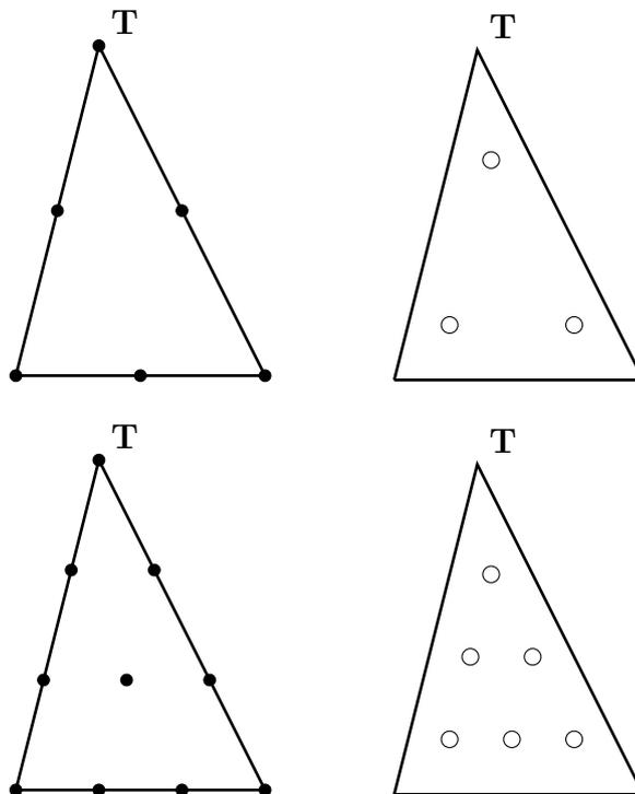
**Figure 4.9:** Elements of the triangulation  $\mathcal{T}_h$  with the local degrees of freedom represented as filled circles for the velocity (left) and with the local degrees of freedom pictured by circles for the pressure (right), for the  $\mathbf{P}_2/P_1^{\text{disc}}$ -element on top and  $\mathbf{P}_3/P_2^{\text{disc}}$ -element beneath.
