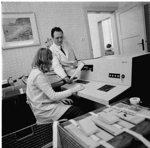
SER2d by VEB Elektronische Rechenmaschinen Karl-Marx-Stadt (around 1962) My secondary school owned one around 1975
