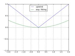
Comparison of artificial diffusion functions  $\frac{1}{2}|x|$  (upwind) and  $\frac{1}{2}|x|+B(|x|)-1$  (exp. fitting)
