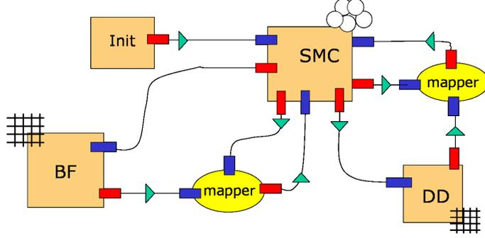
Figure 5. The Connection Scheme, showing the single scale models (Bulk Flow, SMC, Drug Diffusion), the Init agent (used to generate the initial structural stress condition in the tissue), the mapper agents and the conduits. Single scale models are mesh-based (BF, DD) or Agent-based (SMC).
