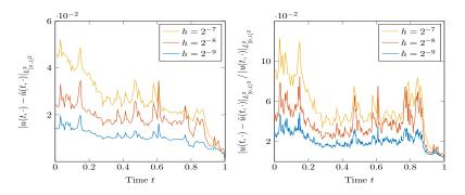
FIGURE 3. Absolute and relative error between RPDE and pseudoregression solution. The parameters are K = 36,  $M = 10^6$  and  $h = 2^{-7}, 2^{-8}, 2^{-9}$ .
