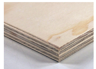
Fig. 2: Plywood consisting of multiple horizontal wooden layers. https://commons.wikimedia.org/wiki/File:Spruce_plywood.JPG
