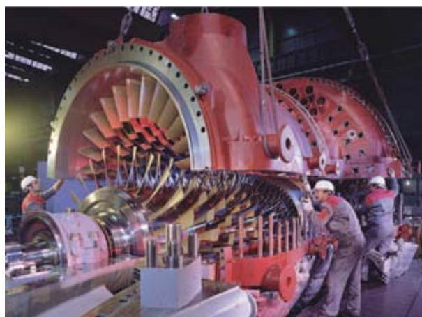
Fig. 1: Assembly of a gas turbine (source: ALSTOM Power Ltd.)
