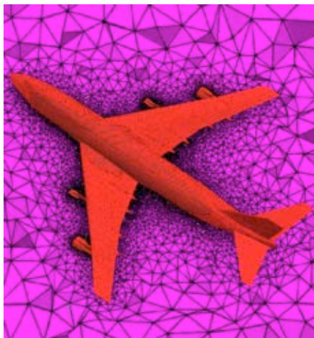
(c) Mesh detail (490,692 nodes and 2,709,770 tetrahedra)
