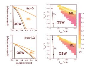
**Fig. 4:** Larger regions with stable mode-locking (ML) for lasers with optimized design (upper figures). Theoretical prediction (left), experiment (right)
