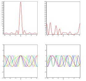
**Fig. 2:** Composition of a pulse by superposition of modes with properly locked phases (left); irregular pattern for a superposition of the same modes with arbitrary phases (right)
