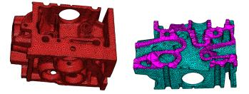
*Fig. 2:* Engine part (IFP, France): geometry, TetGen mesh
