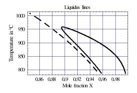
**Fig. 4:** Lines of existence of liquid GaAs. Dashed and solid lines, respectively: liquidus lines without (dashed) and with (solid) mechanical and interfacial energies.
