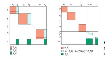
**Fig. 3:** Structure of the Jacobian before and after block Schur complement operation
