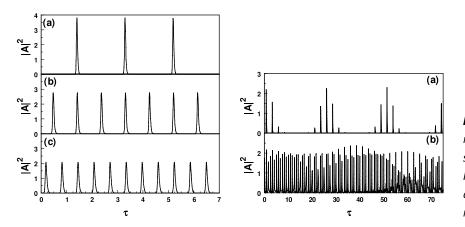
Fig. 3: Dynamical regimes of mode-locked lasers. Left: subharmonic mode-locking. Right: periodically (a) and chaotically (b) modulated mode-locking.
