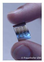
Fig. 6: Micro fuel cell (Fraunhofer IZM)
