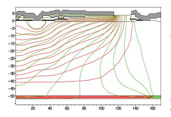
**Fig. 1:** WIAS-TeSCA simulation of the cross section of a transistor: isolines of the electric field. The compression at the transition between contact (Dirichlet boundary) and insulator (Neumann boundary) indicates steep gradients of the electrostatic potential.
