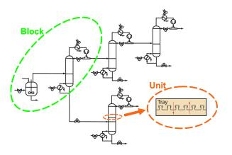
**Fig. 2:** Sample of a user-defined block in a part of a reaction-distillation flowsheet
