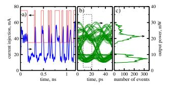
**Fig. 1:** Simulated response of the newly developed laser device under PRBS current modulation. (a): injected current (red), field output (blue). (b): open eye diagram. (c): histogram of points within the dashed box of panel (b). 63
