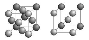
*Fig. 1:* Possible unit lattice cells of steel; left: austenite, right: ferrite.
