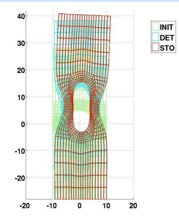
Forward problem: the comparison of the mean values of the total displacement for deterministic, initial and stochastic configuration
