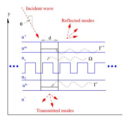
Figure 1: Cross section of grating.
