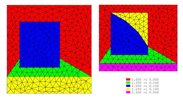
Figure 31: General grating without and with additional interface.
