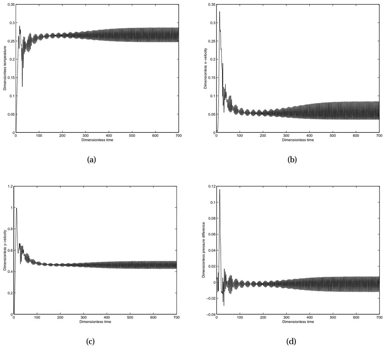
Figure 3: Time histories of dimensionless flow quantities; (a) temperature in point 1; (b) x-velocity component in point 1; (c) y-velocity component in point 1; (d) pressure difference between points 1 and 4.
