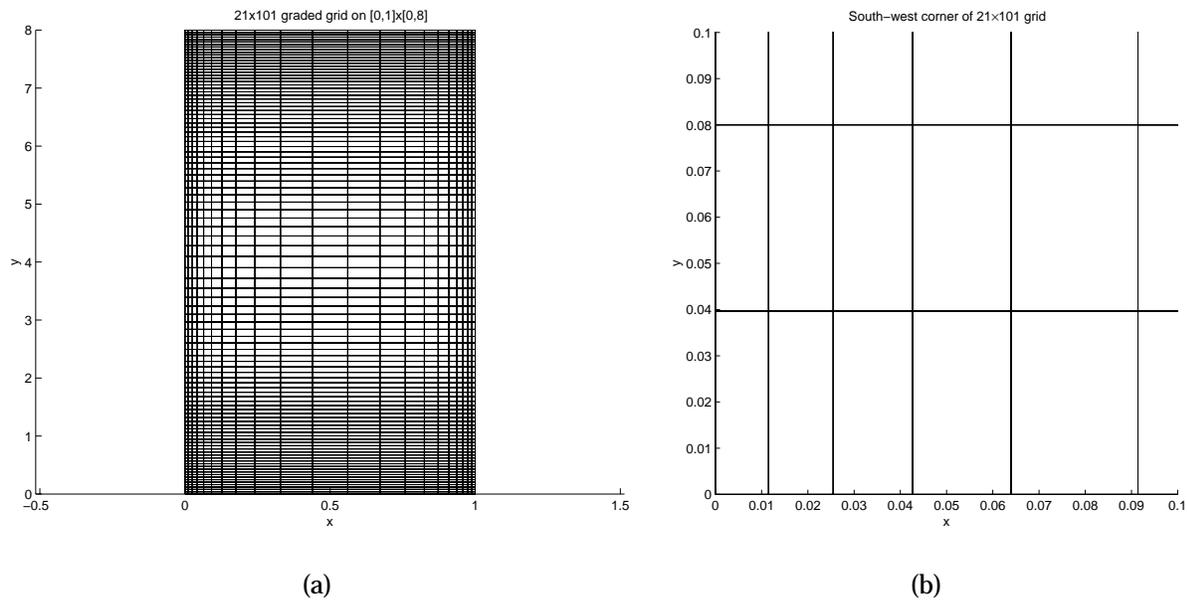
Figure 2: Graded grid of a medium level of refinement; (a) the whole domain; (b) a close-up of the south-west corner.
