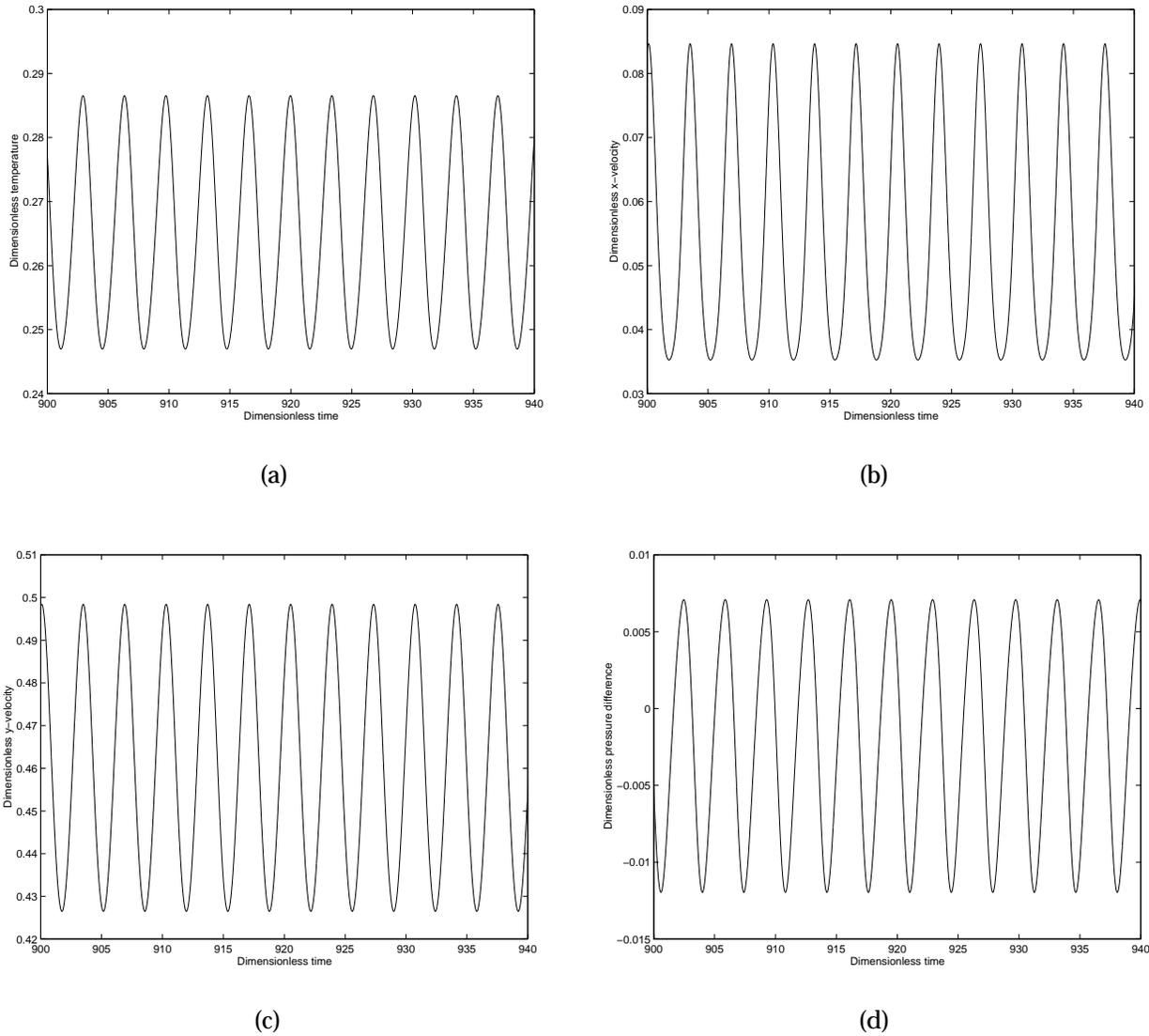
Figure 4: Oscillatory behaviour of flow quantities during periodic phase; (a) temperature in point 1; (b) x-velocity component in point 1; (c) y-velocity component in point 1; (d) pressure difference between points 1 and 4.
