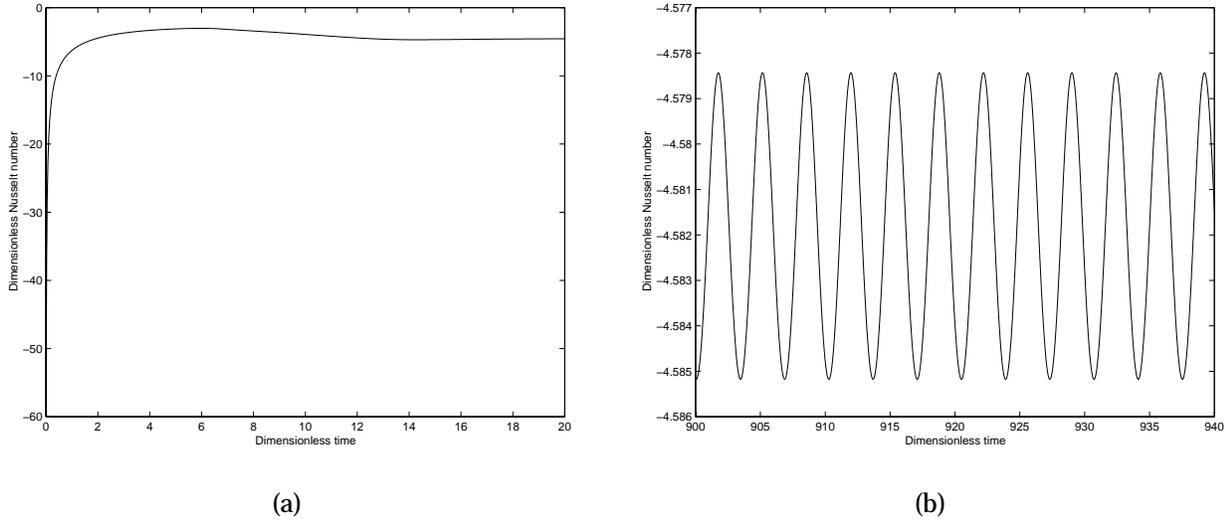
Figure 5: Time history of the Nusselt number on vertical walls: (a) global profile; (b) local oscillatory behaviour during periodic phase.
