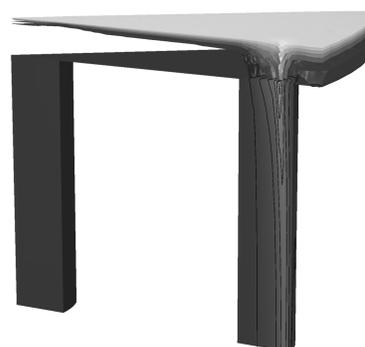
Divergence-free coupling methods allow e.g. to simulate the transport of ions in an electrolyte through a flowcell to validate measurements and determine problem parameters in regimes not covered by the literature. The figure on the left depicts isosurfaces of the ion concentration from [1]. The ultimate goal is to find an efficient discretisation scheme with reasonable complexity.
