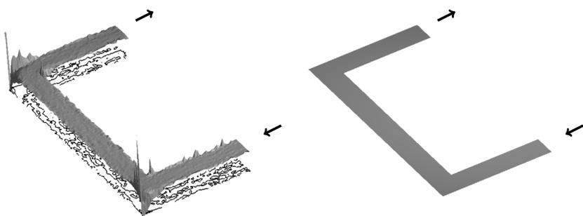
Isolines (on the base) and elevation graph of stationary concentration in the longitudinal section of an U-shaped pipe: standard CR-FEM velocity without reconstruction (left) and with modified CR-FEM velocity (right).
