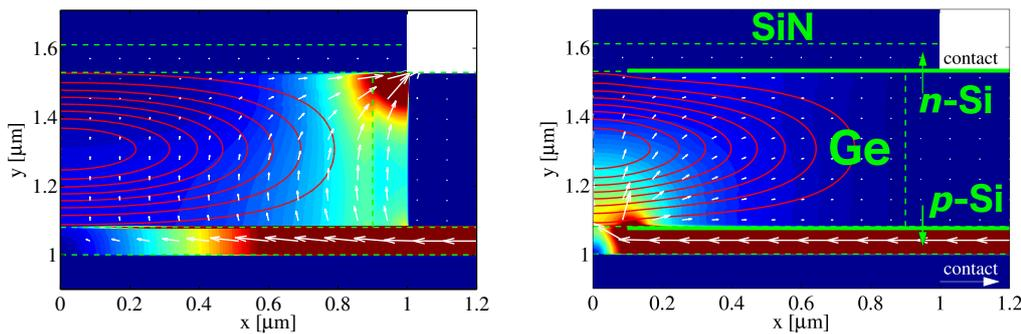
Fig. 7: Hole current for left: standard device and right: aperture device above threshold. Red lines indicate the isolvels of  $\Theta^2$ , whereas the white arrows and the colored background show the direction and magnitude of (the current)  $j_p = -\mu_p p \nabla \phi_p$ .
