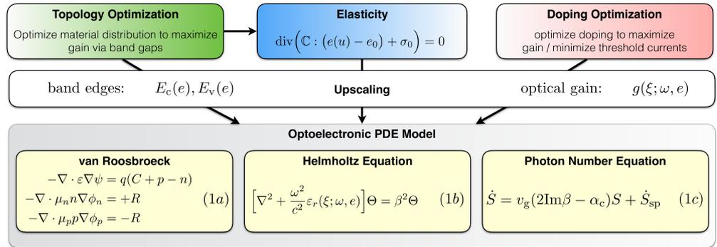
For a semiconductor occupying the domain  $\Omega \subset \mathbb{R}^d$ , charge transport is described by the *van Roosbroeck* system (1a), where, for a given doping profile  $C$ , one seeks the state  $\xi = (\psi, \phi_n, \phi_p)$  consisting of the electric potential  $\psi$ , and the quasi-fermi potentials  $\phi_n, \phi_p$  for electrons and holes. With distribution function  $F$ , the carrier densities  $n, p$  are related to the potentials by
