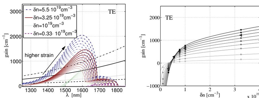
**Fig. 3:** Left: Material gain for TE polarization computed for different excess densities  $\delta n$  and nine linearly increasing biaxial strains 0.35% – 0.7% for Ge with  $n$ -type doping  $C = 5 \cdot 10^{19} \text{ cm}^{-3}$ . Right: Fit to analytic expression for fixed wavelength  $\lambda = 1620 \text{ nm}$ ; see [5].
