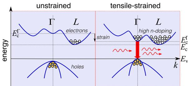
**Fig. 2:** Schematic Ge band structure showing the occupation of electrons and holes in the conduction and valence band. The combined effect of tensile strain and  $n$ -doping resulting in an increase of stimulated emission by reducing the direct band gap  $E_c^\Gamma - E_v$  (strain) and by filling the  $\Gamma$ -band (doping)
