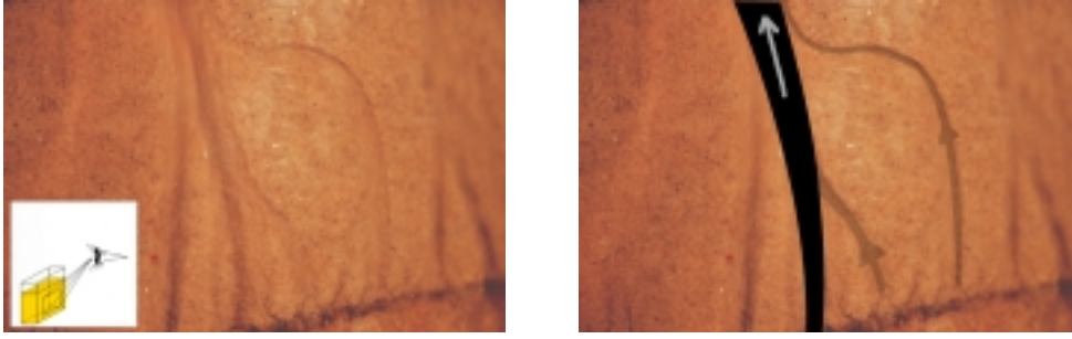
Figure 3: Pipe formation in seepage experiment. Picture from a seepage experiment: At high fluid velocities channels start to select a big channel (marked as a dark shadow on the right) for the flow in the direction to the top, while small channels are reoriented in direction of the big channel (light shadows on the right). The small picture in the box indicates the position of the camera, and the area of the experimental glass container reproduced in pictures.
