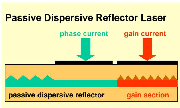
Fig. 1: Scheme of a passive dispersive reflector (PDR) laser. Only the carriers in the gain section couple to the optical field. The waveguide in the PDR sections is passive. The example sketched here consists of a phase tuning section and a DFB-section.
