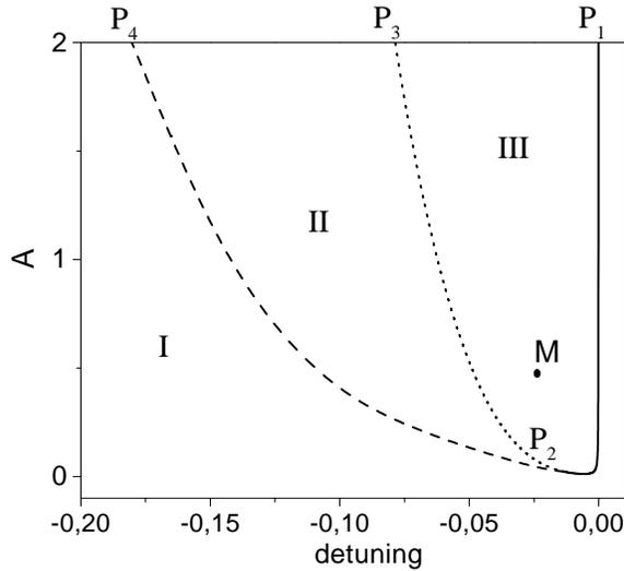
*Fig. 7: Decomposition of the  $(n_0, A)$ -plane in three regions with different qualitative behaviour, where  $W = 0.02$ ,  $\mathcal{J} = 2$  and  $\alpha = 5$ ,  $\Delta = 0.1$*
