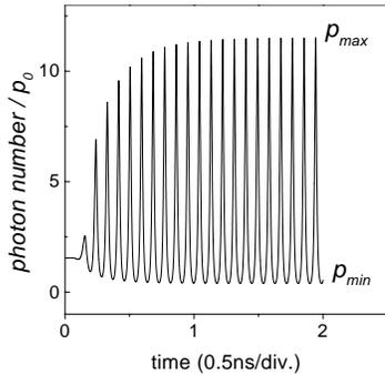
Fig. 5: Time evolution of photon number/ $p_0$  for negative damping and detuning value  $n_{03} = -0.005$  (region of SP), where  $\mathcal{J} = 2$ ,  $W = 0.02$ ,  $A = 1$ ,  $\alpha = 5$ ,  $\Delta = 0.1$ .
