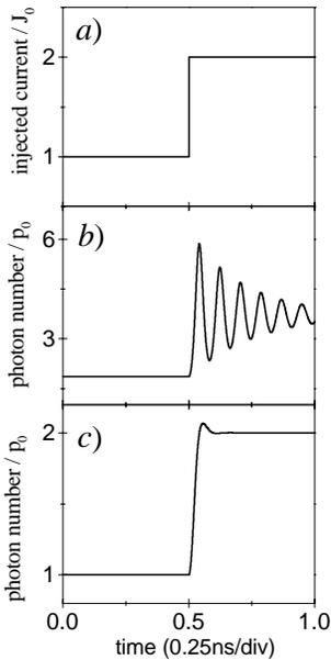
Fig. 4: Time behaviour of the injected current a). Dynamic response of PDRL for different detuning values b)  $n_{01} = 0.05$  (damping of the solitary gain section), c)  $n_{02} = 0.005$  (enhanced damping); where  $W = 0.02$ ,  $A = 1$ ,  $\alpha = 5$ ,  $\Delta = 0.1$ .  $\mathcal{J}_0 = e(N_{th} - N_{tr})/\tau_e$ .
