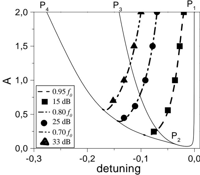
*Fig. 8: Isofrequency contours with  $\alpha = 0$ ,  $W = 0.05$ ,  $\mathcal{J} = 2$ . The bold contours represent curves with the same frequency of self-pulsations. The big marks indicate the same modulation depth. The modulation depth is measured in terms of  $\text{dB} = 10 \log(p_{\max}/p_{\min})$ .*
