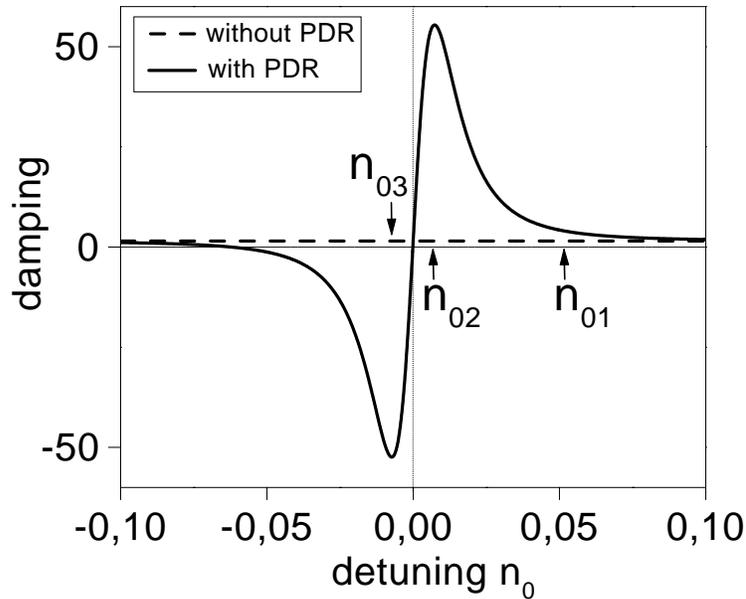
*Fig. 3: Dependence of  $\gamma$  on the detuning  $n_0$  for a solitary gain section (dashed line) and for a gain section with a passive dispersive reflector (solid line) ( $W = 0.02, A = 1, \mathcal{J} = 2$ ).*
