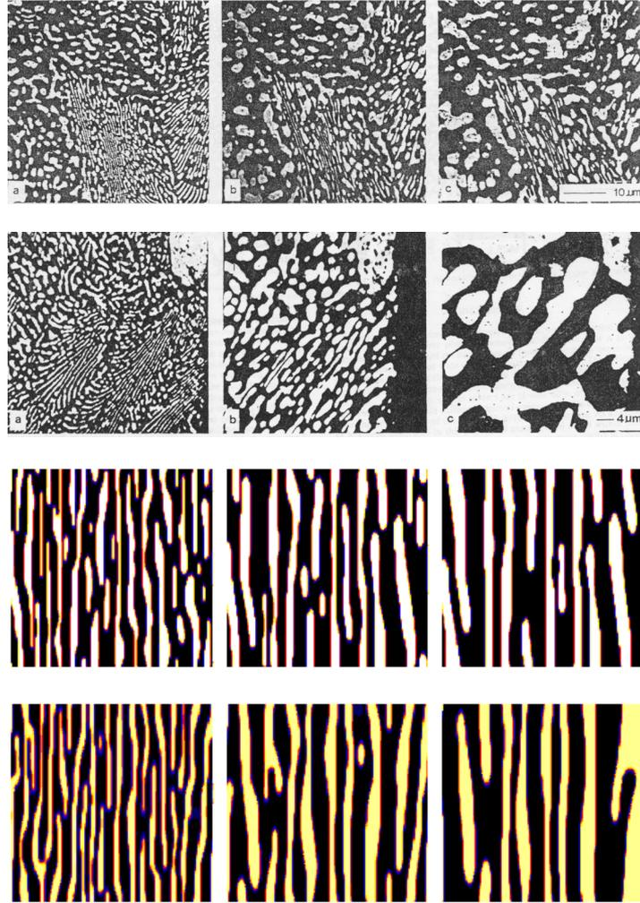
Fig. 4. Comparisons of the coarsening process in SnPb solders: experimental observations vs. and computer simulations (see text).
