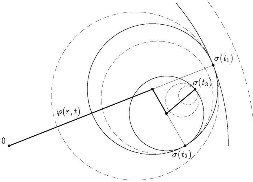
Figure 1: Yield surfaces for a piecewise linear evolution  $t_1 \rightarrow t_2 \rightarrow t_3$  of  $\sigma$ .
