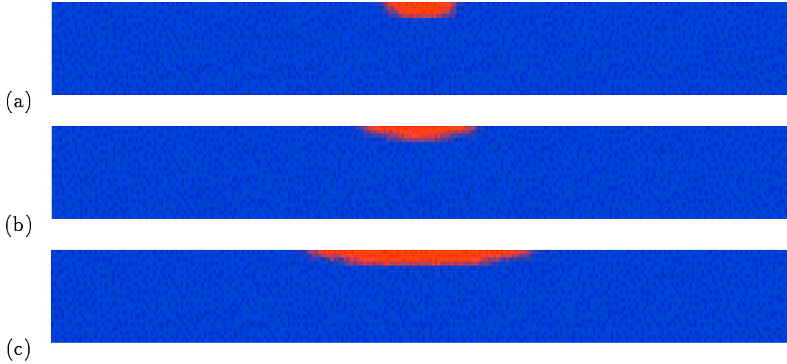
Figure 8: Hardening profile at y = 1.0 , no oscillations; (a) R = 0.25\text{ cm} , v = 150\text{ cm/s} ; (b) R = 0.5\text{ cm} , v = 50\text{ cm/s} ; (c); R = 0.9\text{ cm} , v = 50\text{ cm/s} .
