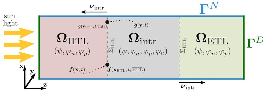
Figure 1: A two-dimensional three-layer device with the relevant potentials stated per subdomain.
