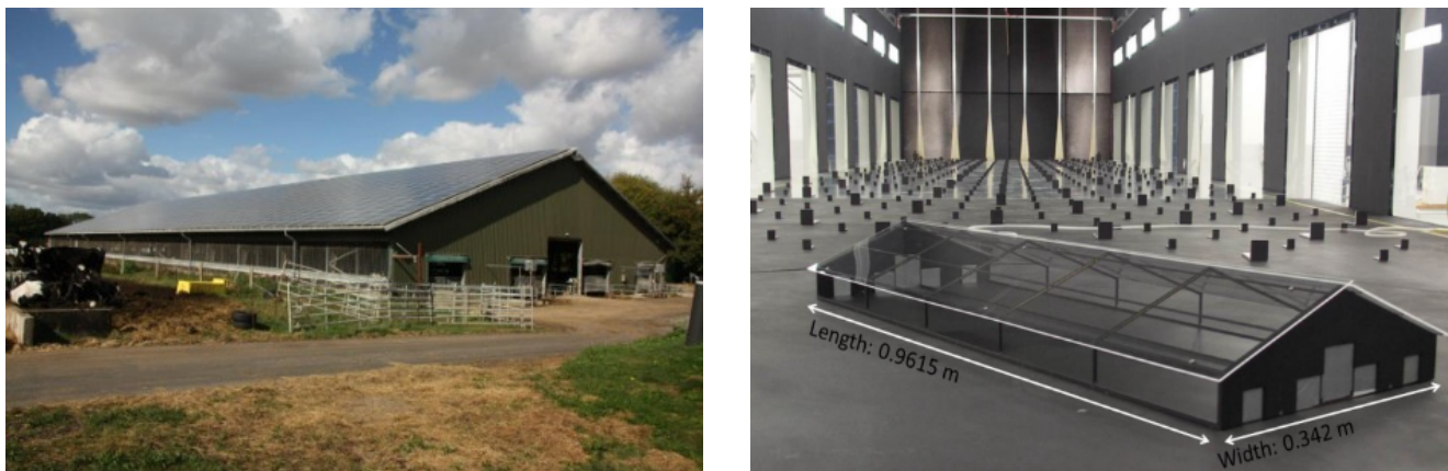
Figure 1: Left: Real scale barn. Right: 1:100 scale model in the wind tunnel.
