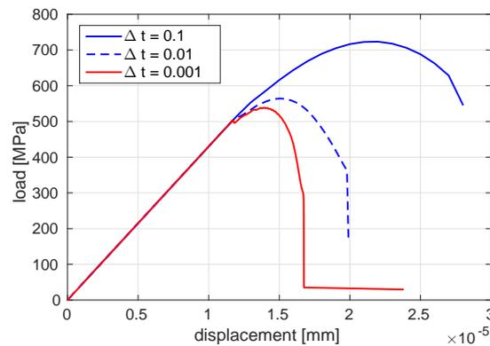
Figure 8: Load-deflection curves for different timestep sizes
