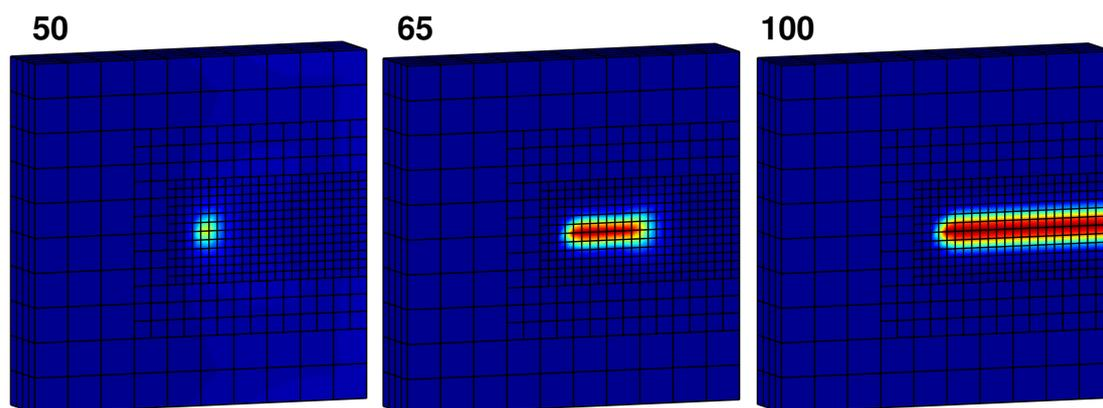
Figure 10: Phase-field snapshots of the mode-I-tension test at different times steps.
