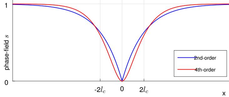
Figure 1: Uniaxial model with a crack at  $x = 0$  and with a continuous phase-field  $s \in [0, 1]$ ; phase-field approximation for a second order and a fourth order approximation of crack density function  $\gamma$ .
