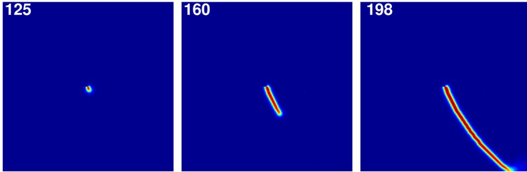
Figure 7: Phase-field snapshots of the mode-II-shear test at different times steps.
