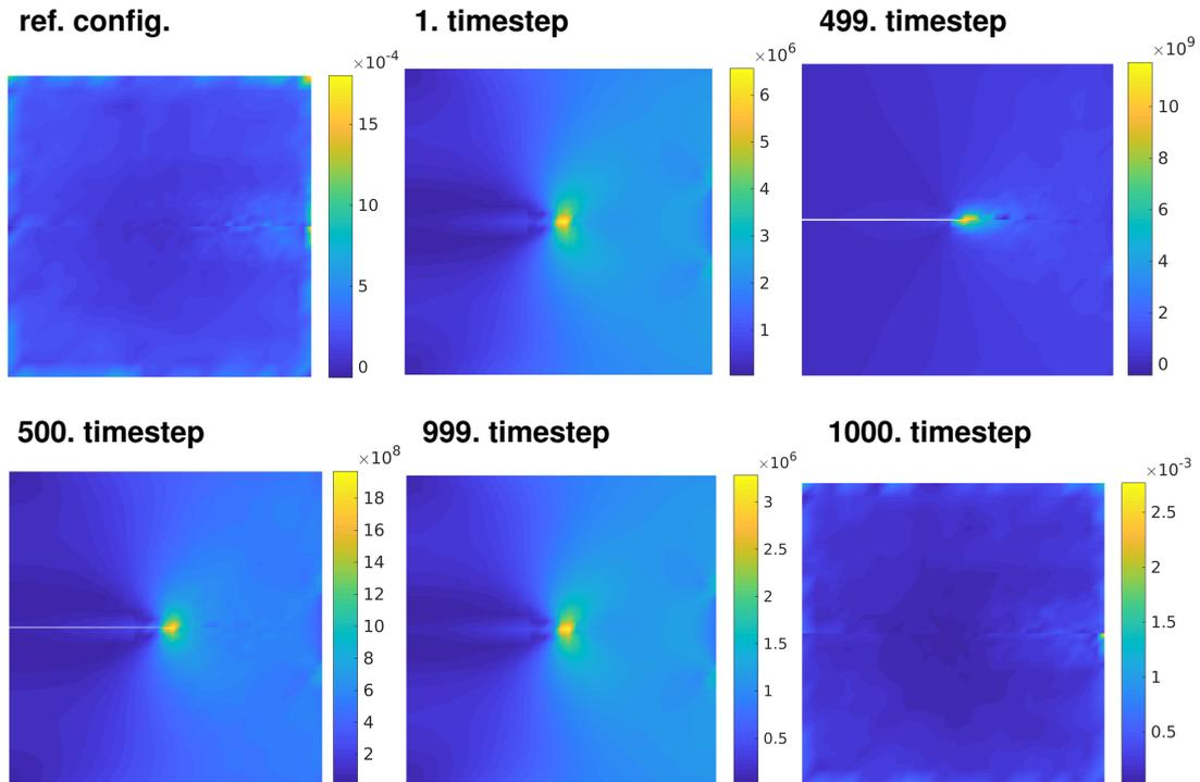
Figure 5: Von Mises stresses of the mode-I-tension test under loading and unloading at different times steps.
