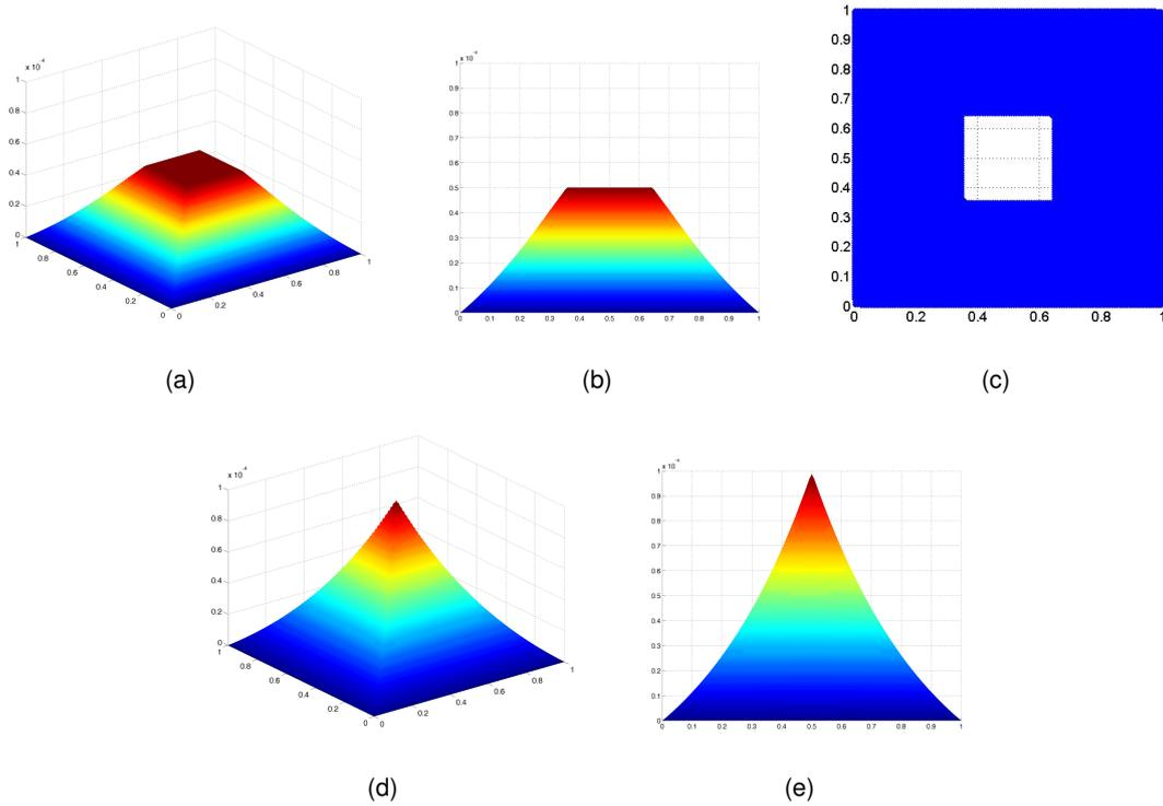
Figure 2: The state  $u(t)$  at time  $t = 5 \times 10^{-5}$  is depicted in figures 2(a), 2(b) and at  $t = 10^{-3}$  in 2(d) and 2(e). The active set  $\mathcal{A}(t)$  at  $t = 5 \times 10^{-5}$  is given in 2(c)
