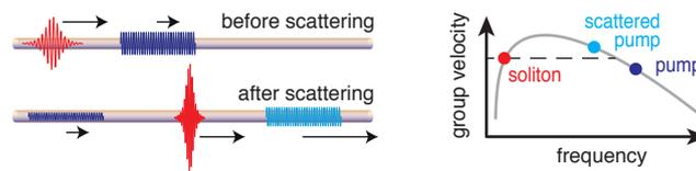
Figure 1: An optical soliton (red) serves as a scatterer for the velocity matched pump wave (blue) and experiences an increase in peak power.
