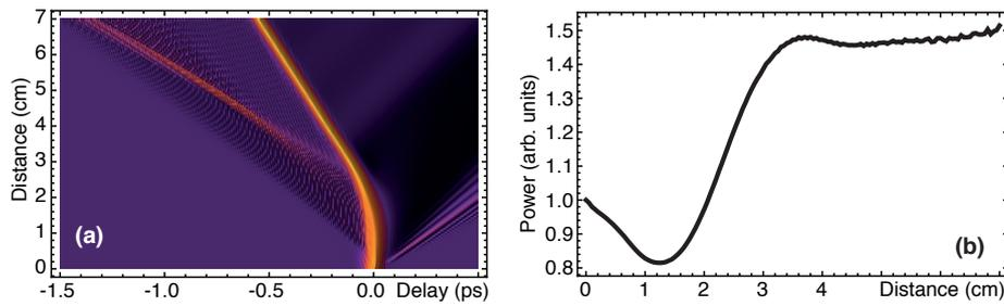
Figure 8: (a) Soliton (2800 nm, FWHM 53 fs) compressed by a continuous pump wave (504 nm, 5% initial solitons peak power). The soliton stabilizes at 2612 nm wavelength and (b) its peak power is amplified by a factor 1.5.
