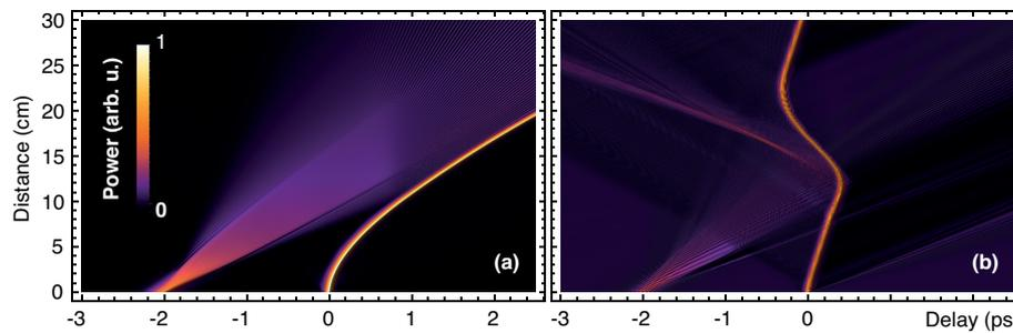
Figure 5: (a) Due to Raman scattering the soliton trajectory (right pulse, 2800 nm, FWHM 53 fs) bends away from the dispersive pulse (left pulse, 504 nm, FWHM 176 fs, 5% of the initial soliton peak power). (b) The soliton trajectory is straightened by an additional low-amplitude continuous pump wave (487 nm, 1.2% of the initial soliton peak power) and interaction with the main pump wave is forced. Soliton peak power is temporarily amplified by a factor 1.3.
