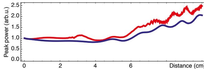
Figure 7: The relative peak power of the compressed fundamental soliton for the calculations shown in Fig. 4a (blue) and Fig. 4b (red). Cancellation of the SSFS leads to an approximately 25% increase of the final peak power.
