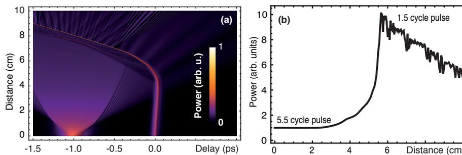
Figure 3: (a) A dispersive wave packet (left pulse, 540 nm, at half maximum (FWHM) 176 fs, and initially 2 times initial soliton power, bulk silica dispersion) is reflected/scattered at a fundamental soliton (right pulse, 2800 nm, 53 fs FWHM). The Raman scattering is artificially switched off. (b) The gain of the soliton peak power is approximately by a factor 10.
