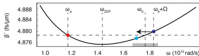
Figure 2: A typical dispersion profile (bulk fused silica) for which a soliton (red point) is effectively compressed by a group velocity matched pump wave (blue point). The pump must belong to the gray domain, which provides a nearly perfect scattering and maximizes energy/momentum transfer. The soliton frequency shift (not shown) is considerably smaller than that of the pump.
