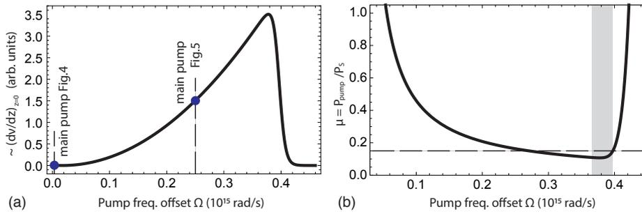
Figure 6: (a) Interval of initial pump frequencies for an effective interaction with a soliton of initial carrier frequency  $\omega_a = 0.67$  PHz (2800 nm wavelength) and FWHM of 53 fs. The maximum of the curve indicates the frequency for the strongest initial influence on the soliton. (b) Pairs of initial pump frequency and amplitude for cancelling the SSFS for a soliton as in (a). The shaded region indicates the parameter region for a stable compensation.
