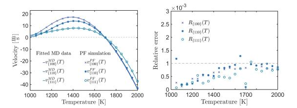
Figure 7: The points in the left figure are the mesured velocities from the numerical solution of equation (11). The solid lines are the fitted velocities from molecular dynamics. Clearly, model (11) with the atomistic informed parameters reproduces exactly the kinetic interace-behavoir. As shown in the right figure, only 5% of the relative errors of the velocities are greater than  $10^{-3}$ . The highest error is about 0.0013 for the {110} orientatin at  $T=1650 {\rm K}$ .
