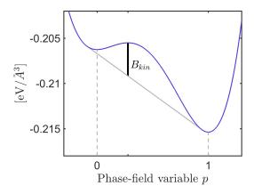
Figure 1: Example of the bulk free energy density F and its kinetic barrier  $B_{kin}$  at temperature 400K (less than  $T_m$ ).  $B_{kin}$  is the kinetic barrier, that has to be overcomed to pass from one phase into the other.
