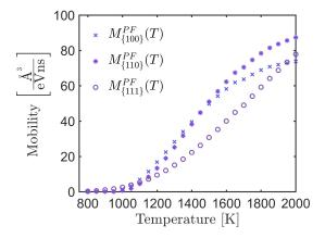
Figure 6: The extracted mobilities of the phase-field model as a function of temperature and orientation. The concrete values are listed in Section A.3 in Table 4.
