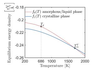
Figure 2: Minimum values for the free energy density for liquid/amorphous  $(f_0(T))$  and crystalline  $(f_1(T))$  equilibrium to the SW potential for a temperature range of 200–2000 K. The free energy equilibrium values are calculated with the codes provided by Ruy and Cai [36]. For the liquid branch,  $T_g$  points out the glass transition. The free energies for the amorphous phase were calculated by Broughton and Li [6].
