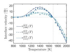
Figure 4: Crystallization velocity over temperature for silicon with the Stillinger-Weber potential, fitted by a Vogel-Fulcher equation(10).
