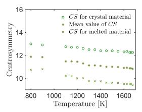
Figure 3: Dependence of the average centrosymmetry parameter of melt and solid on temperature. The mean value  $CS_{crit}(T)$  is used to determine the position of the crystallization front.
