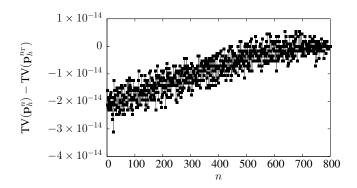
Figure 6: The difference between total variation of the discrete adjoint at time  $t_n$  and total variation of the final time discrete adjoint for Giles' test case.
