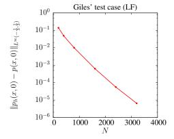
Figure 5: Convergence of the discrete adjoint computed using the Lax-Friedrich method.
