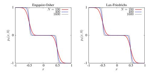
Figure 2: Discrete adjoint computed using Engquist-Osher and Lax-Friedrichs schemes with two-stage TVD-RK method.
