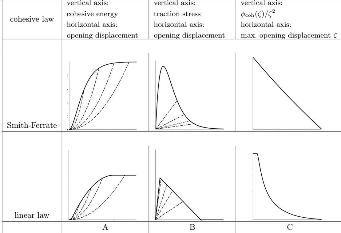
Figure 1: Typical cohesive laws. Solid lines: curves corresponding to maximal loading envelope, dashed lines: loading - unloading rules.
