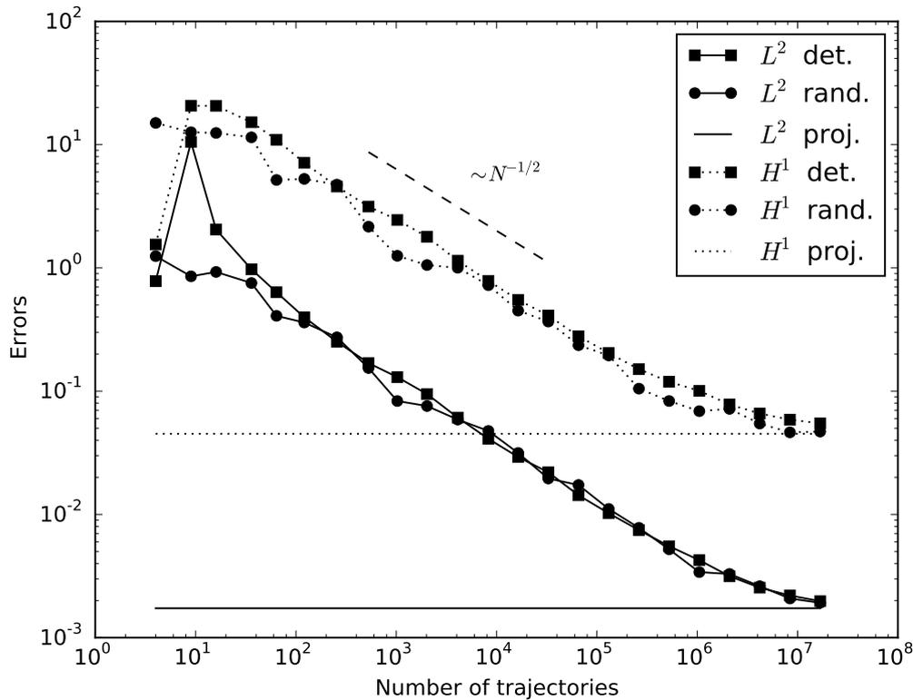
FIGURE 3. The  $L^2$  and  $H^1$  errors from the experiments with deterministic global regression (square) and semi stochastic global regression (circle) on a smooth benchmark field as well as the  $L^2$  and  $H^1$  error of the projection into the polynomial regression space (i.e., the bias, no marker).
