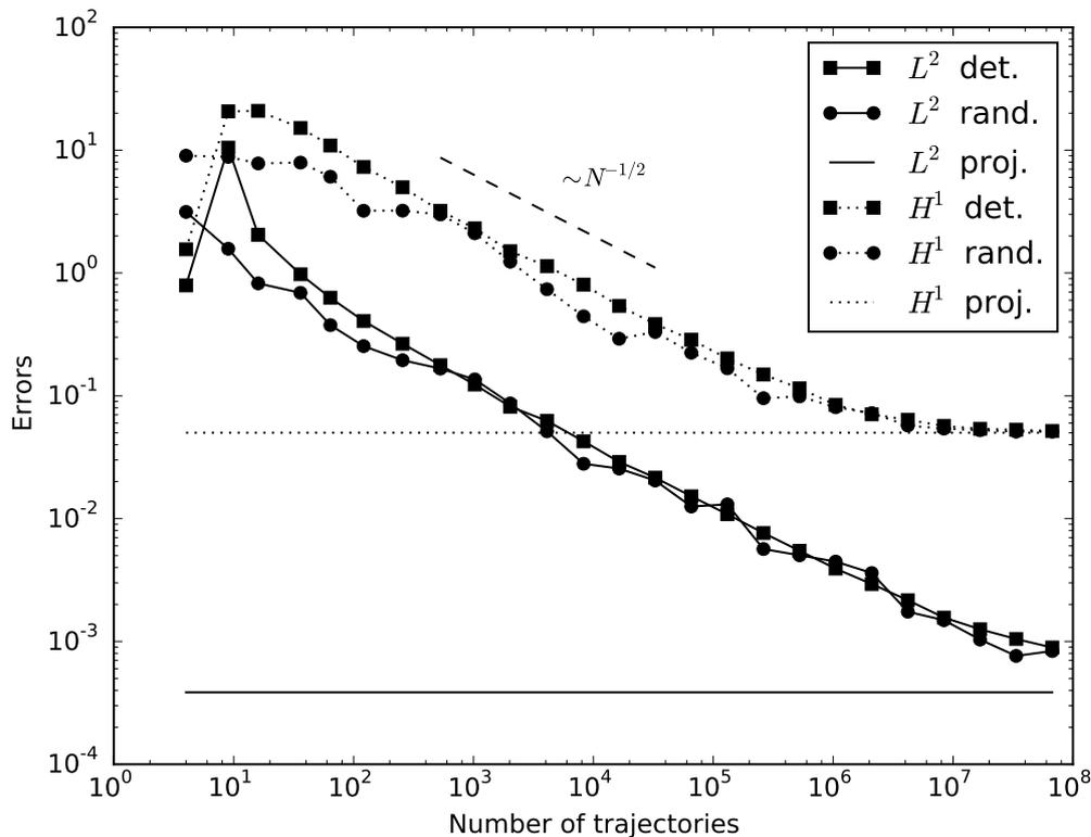
FIGURE 5. The  $L^2$  and  $H^1$  errors from the experiments with deterministic global regression (square) and semi stochastic global regression (circle) on a rough benchmark field as well as the  $L^2$  and  $H^1$  error of the projection into the polynomial regression space (no marker).
