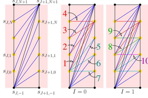
■ **Figure 10** An example of the sequence of edge flips applied on one section of the top triangulations  $\mathcal{T}_t^s$ . Left is the initial triangulation before the edge flips. Right shows the sequence is the newly created edges with their indices by the flip sequence.
