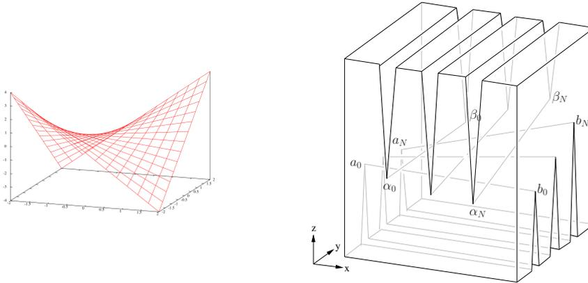
■ **Figure 1** Left: A saddle surface (a hyperbolic paraboloid). Right: The Chazelle polyhedron [4] with three notches, i.e.,  $N = 2$ , on the top and the bottom faces, respectively.
