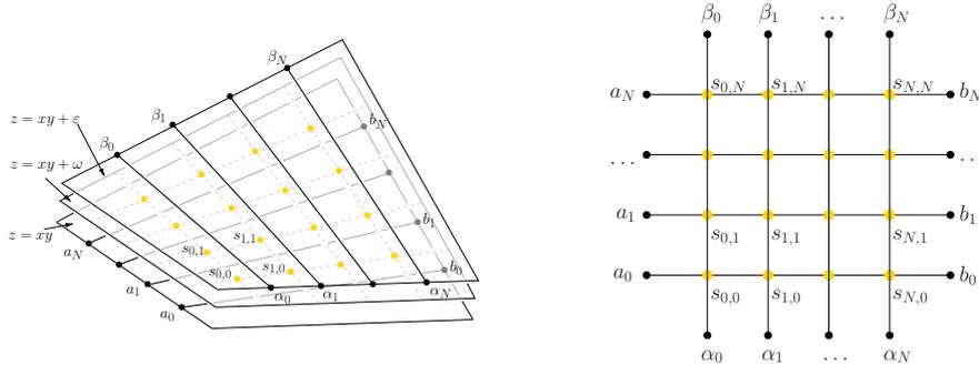
■ **Figure 5** The interior Steiner points,  $\{s_{i,j} \mid i, j = 0, \dots, N\}$ , are placed directly at the intersections of the two set of lines in the  $xy$ -plane and all lie on the saddle surface  $z = xy + \omega$ , where  $0 < \omega < \varepsilon$ .
