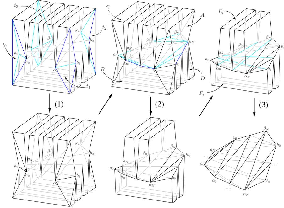
■ **Figure 2** The volume reduction process. The three steps of the reduction are shown by the arrows. It starts from the Chazelle polyhedron (top-left) and ends at the reduced Chazelle polyhedron (bottom-right). At each step, a set of interior edges (shown in blue) is first inserted, and then a number of tetrahedra  $t_1, \dots, t_4$ , and polyhedra:  $A, B, C, D, E_1, \dots, E_N$ , and  $F_1, \dots, F_N$  are removed.
