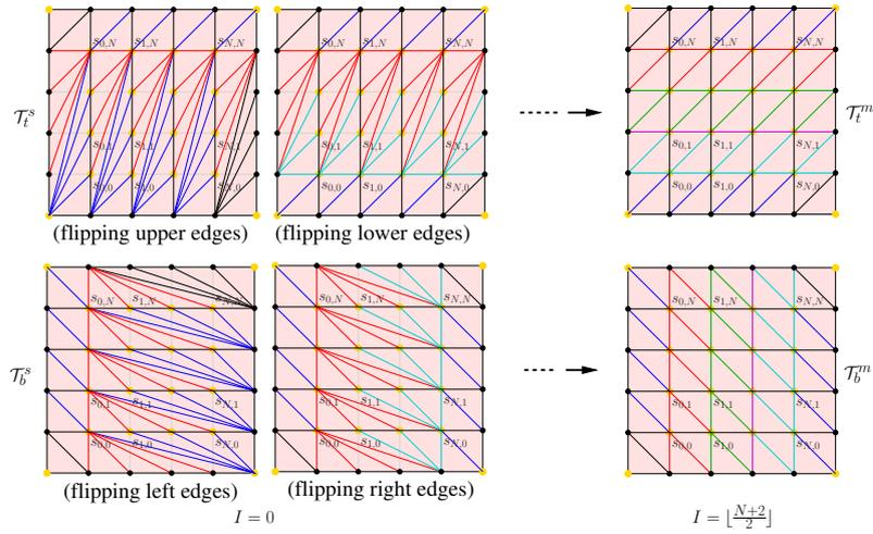
■ **Figure 9** An example result of the second step of the transformation algorithm. Two sequences of edge flips are applied on top and bottom triangulations, respectively. The resulting two triangulations  $\mathcal{T}_t^m$  and  $\mathcal{T}_b^m$  are shown on the right.
