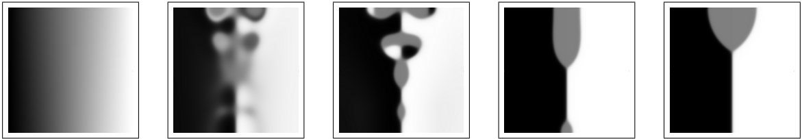
FIGURE 2. Phase separation process in a ternary system for a mirror-symmetric, slightly different initial value. There occur metastable states. Finally, the phases are separated by a straight line and two circular arcs, joining in a triple point. The final state is a global minimizer of the free energy under the constraint of conservation of particle number, see Fig. 3.
