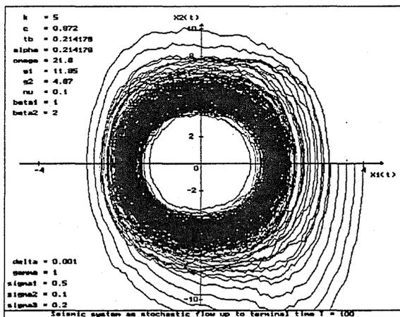
Figure 4: Phase diagram of the nonlinear seismic system with 'critical' build-up time for control force on time interval  $[0, 100]$ .
