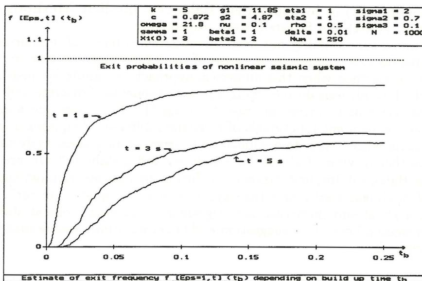
Figure 6: Estimate of the exit frequency  $f_t^e(t_b)$  with varying build-up time  $t_b$  and parameters  $(\gamma, \sigma_1, \sigma_2, \sigma_3, \nu, \beta_1, \beta_2) = (1.0, 2.0, 0.7, 0.1, 0.1, 1.0, 2.0)$  started in  $(3, 0, 0, 0, 0)$  and measured at times  $t = 1, 3, 5$  sec.
