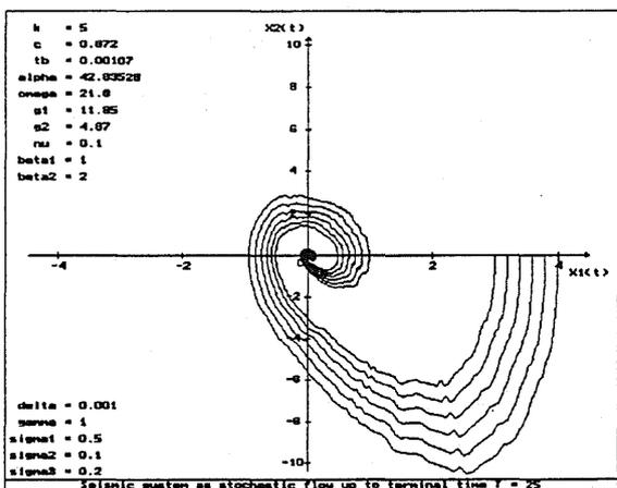
Figure 5: Phase diagram of the nonlinear seismic system with very small build-up time for control force on time interval  $[0, 25]$ .
