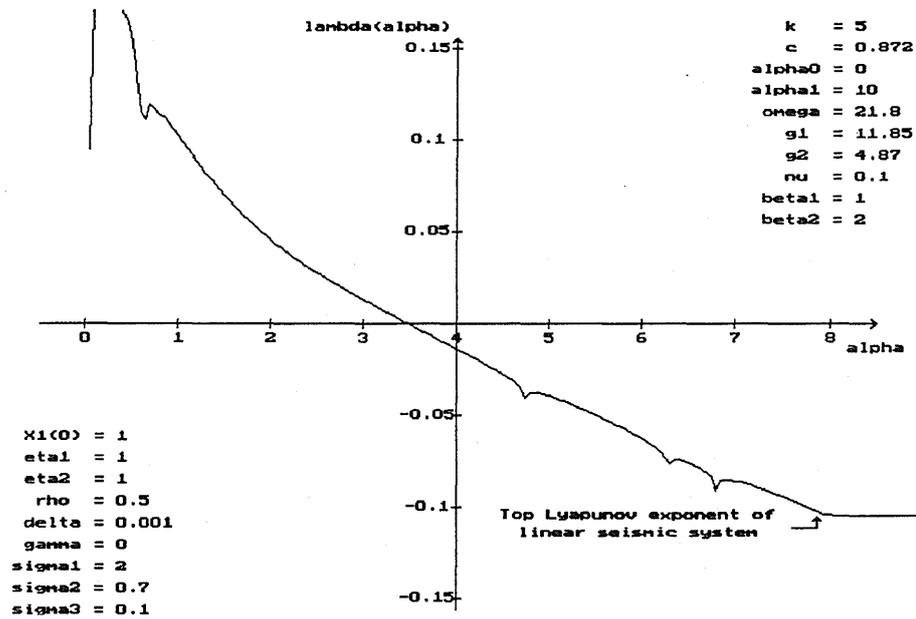
Figure 1: Dependence of the top Lyapunov exponent of the linear system on control speed  $\alpha$  with  $(\gamma, \sigma_1, \sigma_2, \sigma_3, \nu, \beta_1, \beta_2) = (0.0, 2.0, 0.7, 0.1, 0.1, 1.0, 2.0)$  estimated at time  $T = 500$ .
