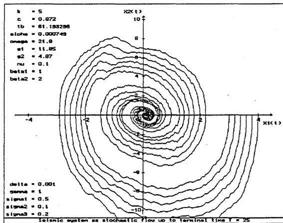
Figure 3: Phase diagram of the nonlinear seismic system with very large build-up time for control force on time interval  $[0, 25]$ .
