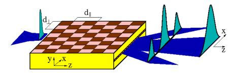
Figure 1: Planar semiconductor amplifier structure with chess-box electrodes. The pump profile is periodically modulated in space, with longitudinal and transverse periods  $d_{\parallel}$  and  $d_{\perp}$ .
