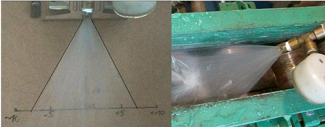
FIGURE 2.1. Jet characteristic of one Lechler nozzle (left) and the water jet in the cooling line (right).
