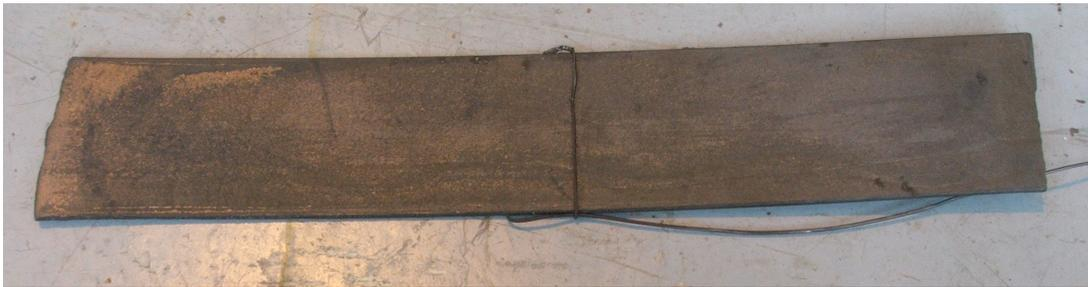
FIGURE 2.3. Sample with thermocouple.
