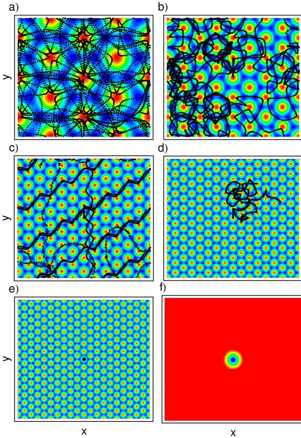
Figure 4: Soliton motion in hexagonal refractive index profiles with different size  $d = 8\pi/(3n)$  of an elementary cell. Here,  $n = 1$  (panel a),  $n = 2$  (b),  $n = 3$  (c),  $n = 4$  (d), and  $n = 5$  (e). The soliton size is approximately visible in panel f).
