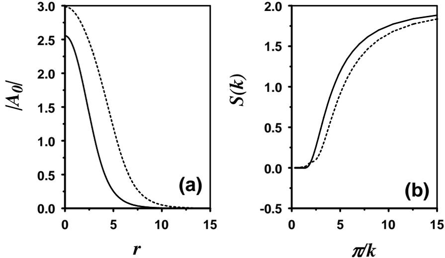
Figure 1: Considered soliton amplitude profiles (a) and the response function  $S(k)$  (b). Solid and dotted lines correspond, respectively, to conservative nonlinearity (2) and dissipative nonlinearity (4) with  $G = 2.11$ ,  $Q = 2.0$ , and  $s = 10$ .
