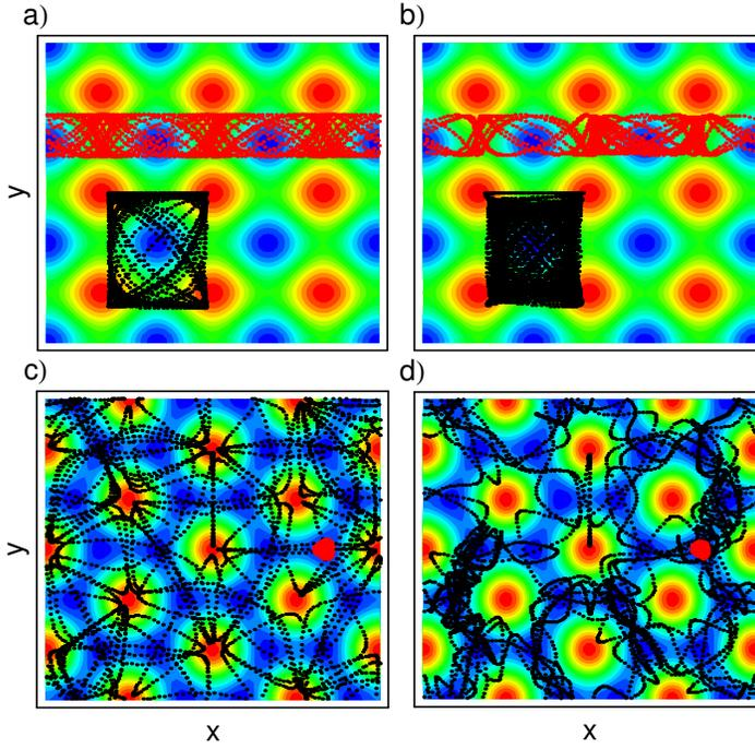
Figure 2: Regular and chaotic soliton motion (black and red curves) in the refractive index profile forming square (a,b) and hexagonal (c,d) lattice. Blue (red) color indicates higher (lower) values of the refractive index. The left two figures (a,c) correspond to conservative nonlinearity (2) and the right two figures (b,d) – to dissipative nonlinearity (4) with the parameter values given in the caption of Fig. 1.
