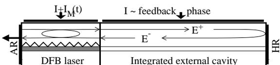
Figure 1: Scheme of the DFB laser with integrated external cavity.
