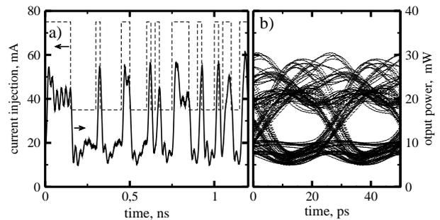
Figure 4: Simulated response of the device to a PRBS current modulation. a): injected current (dashed) and field output (solid). b): open eye diagram.
